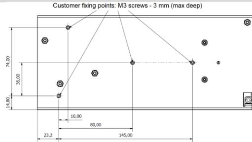
0.7 ÷ 0.8 Nm recommended fixing torque force for M3 screws.
