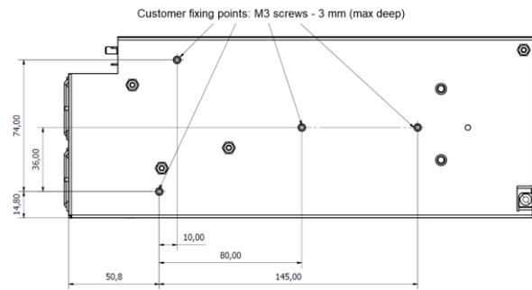
0.7 ÷ 0.8 Nm recommended fixing torque force for M3 screws.
