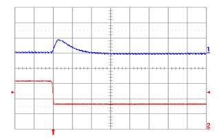
Fig. 1.5V.7: Output voltage response for Vout = 1.5 V to negative load current step change from 16 A to 8 A with slew rate of -5 A/μs at Vin = 12 V. Top trace: output voltage (200 mV/div.); Bottom trace: load current (5 A/div.). Co = 100 μF ceramic. Time scale: 20 μs/div.
