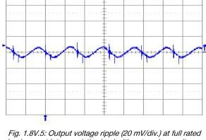
Fig. 1.8V.5: Output voltage ripple (20 mV/div.) at full rated load current into a resistive load with external capacitance 100 μF ceramic and Vin = 12 V for Vout = 1.8 V. Time scale: 2 μs/div.
