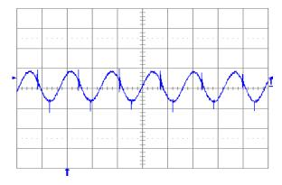
Fig. 3.3V.5: Output voltage ripple (20 mV/div.) at full rated load current into a resistive load with external capacitance  $100 \, \mu F$  ceramic and  $Vin = 12 \, V$  for  $Vout = 3.3 \, V$ . Time scale:  $2 \, \mu s$ /div.
