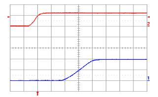
Fig. 2.0V.4: Turn-on transient for Vout = 2.0 V with application of Vin at full rated load current (resistive) and 100 μF external capacitance at Vin = 12 V. Top trace: Vin (10 V/div.); Bottom trace: output voltage (1 V/div.); Time scale: 2 ms/div.
