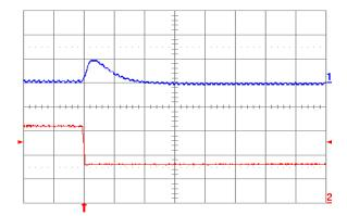
Fig. 1.8V.7: Output voltage response for Vout = 1.8 V to negative load current step change from 16 A to 8 A with slew rate of -5 A/μs at Vin = 12 V. Top trace: output voltage (200 mV/div.); Bottom trace: load current (5 A/div.). Co = 100 μF ceramic. Time scale: 20 μs/div.
