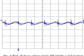
Fig. 1.0V.5: Output voltage ripple (20 mV/div.) at full rated load current into a resistive load with external capacitance  $100 \,\mu\text{F}$  ceramic and  $Vin = 12 \,V$  for  $Vout = 1.0 \,V$ . Time scale:  $2 \,\mu\text{s/div}$ .
