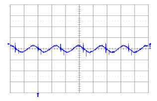
Fig. 1.5V.5: Output voltage ripple (20 mV/div.) at full rated load current into a resistive load with external capacitance 100 μF ceramic and Vin = 12 V for Vout = 1.5 V. Time scale: 2 μs/div.
