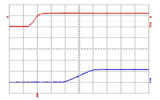
Fig. 1.2V.4: Turn-on transient for Vout = 1.2 V with application of Vin at full rated load current (resistive) and 100 μF external capacitance at Vin = 12 V. Top trace: Vin (10V/div.); Bottom trace: output voltage (1 V/div.); Time scale: 2 ms/div.
