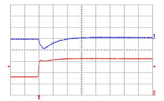
Fig. 1.2V.6: Output voltage response for Vout = 1.2 V to positive load current step change from 8 A to 16 A with slew rate of 5 A/μs at Vin = 12 V. Top trace: output voltage (200 mV/div.); Bottom trace: load current (5 A/div.). Co = 100 μF ceramic. Time scale: 20 μs/div.
