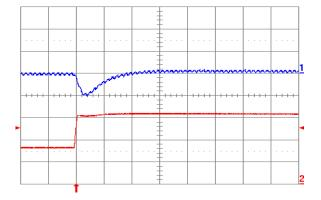
Fig. 2.5V.6: Output voltage response for Vout = 2.5 V to positive load current step change from 8 A to 16 A with slew rate of 5 A/μs at Vin = 12 V. Top trace: output voltage (200 mV/div.); Bottom trace: load current (5 A/div.). Co = 100 μF ceramic. Time scale: 20 μs/div.
