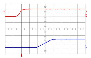
Fig. 0.7525V.4: Turn-on transient for Vout = 0.7525 V with application of Vin at full rated load current (resistive) and 100 μF external capacitance at Vin = 12 V. Top trace: Vin (10 V/div.); Bottom trace: output voltage (0.5 V/div.); Time scale: 2 ms/div.
