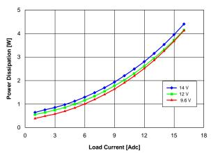
Fig. 1.8V.3: Power loss vs. load current and input voltage for Vout = 1.8 V converter mounted vertically with air flowing at a rate of 200 LFM (1 m/s) and Ta = 25 °C.
