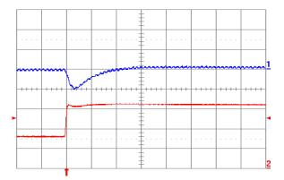
Fig. 1.8V.6: Output voltage response for Vout = 1.8 V to positive load current step change from 8 A to 16 A with slew rate of 5 A/μs at Vin = 12 V. Top trace: output voltage (200 mV/div.); Bottom trace: load current (5 A/div.). Co = 100 μF ceramic. Time scale: 20 μs/div.
