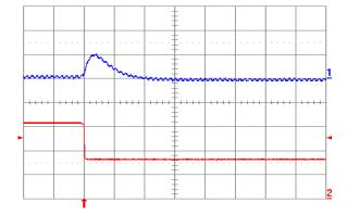
Fig. 2.5V.7: Output voltage response for Vout = 2.5 V to negative load current step change from 16 A to 8 A with slew rate of -5 A/μs at Vin = 12 V. Top trace: output voltage (200 mV/div.); Bottom trace: load current (5 A/div.). Co = 100 μF ceramic. Time scale: 20 μs/div.
