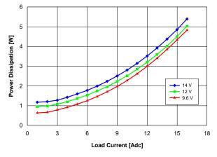
Fig. 5.0V.3: Power loss vs. load current and input voltage for Vout = 5.0 V converter mounted vertically with air flowing at a rate of 200 LFM (1 m/s) and Ta = 25 °C.
