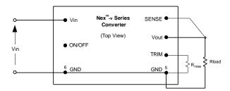
Fig. C: Configuration for programming output voltage.
