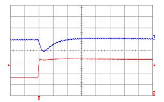
Fig. 2.0V.6: Output voltage response for Vout = 2.0 V to positive load current step change from 8 A to 16 A with slew rate of 5 A/μs at Vin = 12 V. Top trace: output voltage (200 mV/div.); Bottom trace: load current (5 A/div.). Co = 100 μF ceramic. Time scale: 20 μs/div.
