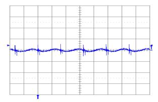
Fig. 0.7525V.5: Output voltage ripple (20 mV/div.) at full rated load current into a resistive load with external capacitance 100 μF ceramic and Vin = 12 V for Vout = 0.7525 V. Time scale: 2 μs/div.
