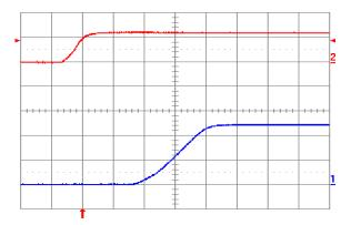
Fig. 2.5V.4: Turn-on transient for Vout = 2.5 V with application of Vin at full rated load current (resistive) and 100 μF external capacitance at Vin = 12 V. Top trace: Vin (10 V/div.); Bottom trace: output voltage (1 V/div.); Time scale: 2 ms/div.
