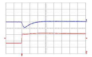
Fig. 1.5V.6: Output voltage response for Vout = 1.5 V to positive load current step change from 8 A to 16 A with slew rate of 5 A/μs at Vin = 12 V. Top trace: output voltage (200 mV/div.); Bottom trace: load current (5 A/div.). Co = 100 μF ceramic. Time scale: 20 μs/div.
