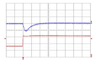
Fig. 3.3V.6: Output voltage response for Vout = 3.3 V to positive load current step change from 8 A to 16 A with slew rate of 5 A/μs at Vin = 12 V. Top trace: output voltage (200 mV/div.); Bottom trace: load current (5 A/div.). Co = 100 μF ceramic. Time scale: 20 μs/div.
