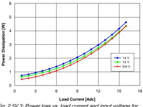
Fig. 2.5V.3: Power loss vs. load current and input voltage for Vout = 2.5 V converter mounted vertically with air flowing at a rate of 200 LFM (1 m/s) and Ta = 25 °C.
