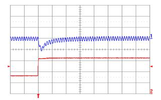
Fig. 5.0V.6: Output voltage response for Vout = 5.0 V to positive load current step change from 8A to 16A with slew rate of 5 A/μs at Vin = 12 V. Top trace: output voltage (200 mV/div.); Bottom trace: load current (5 A/div.). Co = 100 μF ceramic. Time scale: 20 μs/div.
