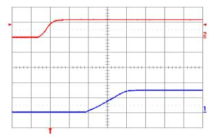
Fig. 1.5V.4: Turn-on transient for Vout = 1.5 V with application of Vin at full rated load current (resistive) and 100 μF external capacitance at Vin = 12 V. Top trace: Vin (10 V/div.); Bottom trace: output voltage (1 V/div.); Time scale: 2 ms/div.
