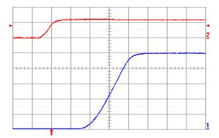
Fig. 5.0V.4: Turn-on transient for Vout = 5.0 V with application of Vin at full rated load current (resistive) and 100 μF external capacitance at Vin = 12 V. Top trace: Vin (10 V/div.); Bottom trace: output voltage (1 V/div.); Time scale: 2 ms/div.
