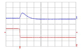
Fig. 1.2V.7: Output voltage response for Vout = 1.2 V to negative load current step change from 16 A to 8 A with slew rate of -5 A/μs at Vin = 12 V. Top trace: output voltage (200 mV/div.); Bottom trace: load current (5 A/div.). Co = 100 μF ceramic. Time scale: 20 μs/div.
