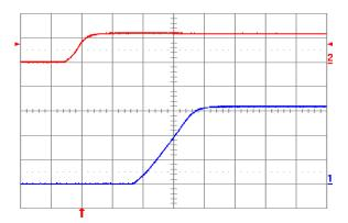
Fig. 3.3V.4: Turn-on transient for Vout = 3.3 V with application of Vin at full rated load current (resistive) and 100 μF external capacitance at Vin = 12 V. Top trace: Vin (10 V/div.); Bottom trace: output voltage (1 V/div.); Time scale: 2 ms/div.
