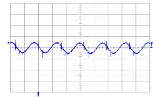
Fig. 2.0V.5: Output voltage ripple (20 mV/div.) at full rated load current into a resistive load with external capacitance  $100 \, \mu F$  ceramic and  $Vin = 12 \, V$  for  $Vout = 2.0 \, V$ . Time scale:  $2 \, \mu s/div$ .
