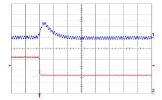
Fig. 5.0V.7: Output voltage response for Vout = 5.0 V to negative load current step change from 16 A to 8 A with slew rate of -5 A/μs at Vin = 12 V. Top trace: output voltage (200 mV/div.); Bottom trace: load current (5 A/div.). Co = 100 μF ceramic. Time scale: 20 μs/div.
