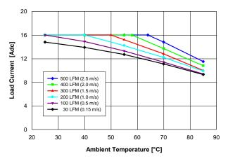
Fig. 5.0V.1: Available load current vs. ambient temperature and airflow rates for Vout = 5.0 V converter mounted vertically with Vin = 12 V, and maximum MOSFET temperature  $\leq 120 \text{ °C}$ .
