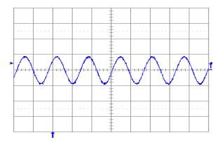
Fig. 5.0V.5: Output voltage ripple (20 mV/div.) at full rated load current into a resistive load with external capacitance  $100 \, \mu F$  ceramic and  $Vin = 12 \, V$  for  $Vout = 5.0 \, V$ . Time scale:  $2 \, \mu s$ /div.
