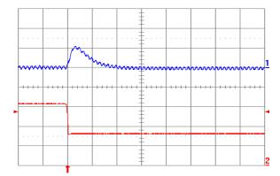
Fig. 3.3V.7: Output voltage response for Vout = 3.3 V to negative load current step change from 16 A to 8 A with slew rate of -5 A/μs at Vin = 12 V. Top trace: output voltage (200 mV/div.); Bottom trace: load current (5 A/div.). Co = 100 μF ceramic. Time scale: 20 μs/div.
