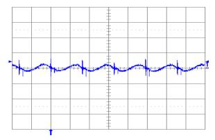
Fig. 1.2V.5: Output voltage ripple (20 mV/div.) at full rated load current into a resistive load with external capacitance  $100\,\mu\text{F}$  ceramic and  $Vin = 12\,V$  for  $Vout = 1.2\,V$ . Time scale:  $2\,\mu\text{s}/\text{div}$ .
