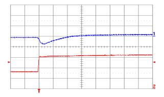
Fig. 0.7525V.6: Output voltage response for Vout = 0.7525 V to positive load current step change from 8 A to 16 A with slew rate of 5 A/μs at Vin = 12 V. Top trace: output voltage (200 mV/div.); Bottom trace: load current (5 A/div.). Co = 100 μF ceramic. Time scale: 20 μs/div.
