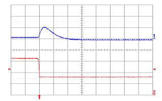
Fig. 1.0V.7: Output voltage response for Vout = 1.0 V to negative load current step change from 16 A to 8 A with slew rate of -5 A/μs at Vin = 12 V. Top trace: output voltage (200 mV/div.); Bottom trace: load current (5 A/div.). Co = 100 μF ceramic. Time scale: 20 μs/div.
