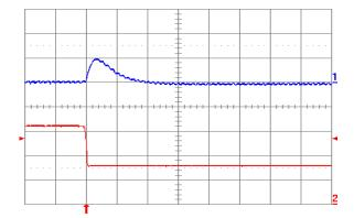
Fig. 2.0V.7: Output voltage response for Vout = 2.0 V to negative load current step change from 16 A to 8 A with slew rate of -5 A/μs at Vin = 12 V. Top trace: output voltage (200 mV/div.); Bottom trace: load current (5 A/div.). Co = 100 μF ceramic. Time scale: 20 μs/div.
