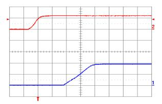
Fig. 1.0V.4: Turn-on transient for Vout = 1.0 V with application of Vin at full rated load current (resistive) and 100  $\mu$ F external capacitance at Vin = 12 V. Top trace: Vin (10 V/div.); Bottom trace: output voltage (0.5 V/div.); Time scale: 2 ms/div.
