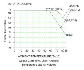
Figure 34. Thermal derating curve @ Vin = 24 V
