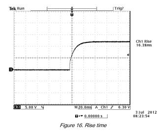
Test Condition: Vin = 48 V, Full Load.
