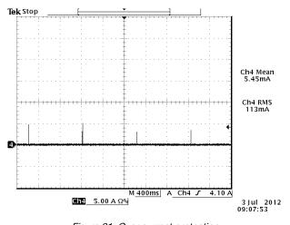
Figure 21. Over current protection Test condition: Vin = 48 V. Full Load
