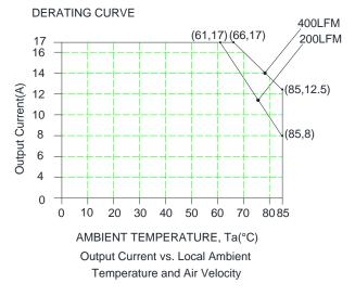
Figure 33. Thermal derating curve @ Vin = 18 V
