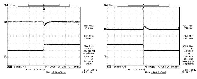
Figure 14. Vout = 12 V, 25%-50% Load Transients at Vin = 48 V @ Ta = 25 °C
