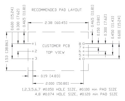
Figure 43. Recommended pad layout
