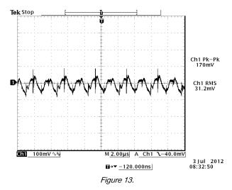
Note: Ripple and noise, 48 VDC input, 17 A output, Ta = 25 °C, with 1 µF ceramic and 10 µF Tan cap.
