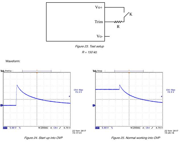
CH1: Output voltage waveform
