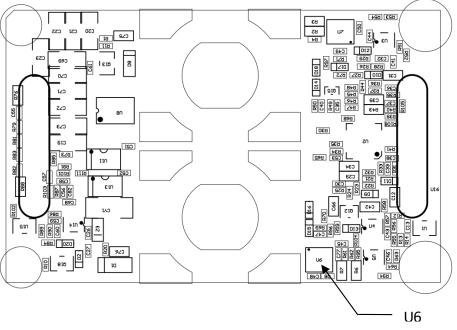
Figure 26. Temperature reference points on bottom side
