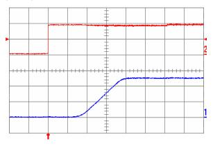
Fig. 2.5V.7: Output voltage response (YNL05S10025) to positive load current step change from 5 A to 10 A with slew rate of 5 A/ $\mu$ s at Vin = 5 V. Top trace: output voltage 47  $\mu$ F ceramic + 1  $\mu$ F ceramic. Time scale: 20  $\mu$ s/div.
