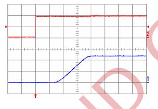
Fig. 1.2V.6: Output voltage response (YNL05S10012) to positive load current step change from 5 A to 10 A with slew rate of 5 A/ $\mu$ s at Vin = 5 V. Top trace: output voltage (100 mV/div.); Bottom trace: load current (5 A/div.). Co = 47  $\mu$ F ceramic + 1  $\mu$ F ceramic. Time scale: 20  $\mu$ s/div.
