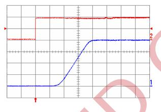
Fig. 2.0V.7: Output voltage response (YNL05S10020) to positive load current step change from 5 A to 10 A with slew rate of 5 A/ $\mu$ s at Vin = 5 V. Top trace: output voltage (100 mV/div.); Bottom trace: load current (5 A/div.). Co = 47  $\mu$ F ceramic + 1  $\mu$ F ceramic. Time scale: 20  $\mu$ s/div.
