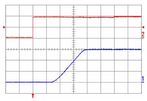
Fig. 1.5V.7: Output voltage response (YNL05S10015) to positive load current step change from 5 A to 10 A with slew rate of 5 A/ $\mu$ s at Vin = 5 V. Top trace: output voltage (100 mV/div.); Bottom trace: load current (5 A/div.). Co = 47  $\mu$ F ceramic + 1  $\mu$ F ceramic. Time scale: 20  $\mu$ s/div.
