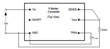
To trim up the output voltage, refer to Fig. E.A trim resistor,  $R_{T-INCR}$ , should be connected between TRIM pin (Pin 3) and GND pin (Pin 5) with value of:
