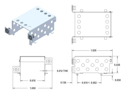
All dimensions in inches. All dimensions +- 0.005", unless noted Screw torque 0.50 +/- 0.10 in-lbs
