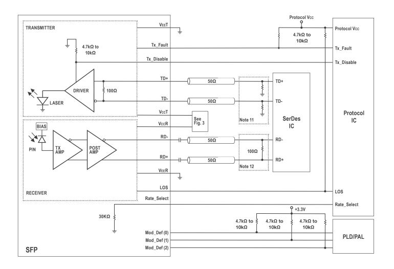
Figure 1 Illustrates the recommended transmit and receive data line terminations.
