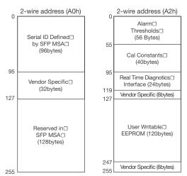
Figure 3 Digital diagnostic memory map specific data field descriptions.
