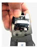
To remover the die set from the hand tool frame loosen thumb Screw (C) completely. Close Ratcheted tool handle one click to reveal the Cap head screw (D). With the opening (E) (approximately .28"), push the die set out from the opposite side.
