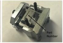
Carefully remove the blade with the springs attached by sliding blade over the alignment pins. When inserting new blade make sure the part number side of the blade is visible before installing cover plate. Re-install cover plate, springs and acorn nuts. Make sure everything moves freely before inserting die set into hand tool frame.
