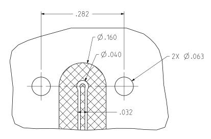
RECOMMENDED PCB LAYOUT NOTE: THIS PATTERN IS FOR REFERENCE ONLY. PATTERN MAY VARY DEPENDING ON ASSEMBLY PROCESS, BOARD TYPE, OR SPECIFIC ELECTRICAL OR MECHANICAL REQUIREMENTS.
