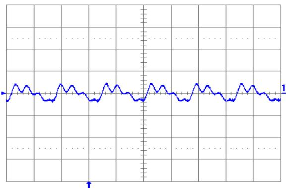
Fig. 2.0V.5: Output voltage ripple (20mV/div.) at full rated load current into a resistive load with external capacitance  $100\text{ }\mu\text{F}$  ceramic +  $1\text{ }\mu\text{F}$  ceramic and  $V_{in} = 12\text{ V}$  for  $V_{out} = 2.0\text{ V}$ . Time scale: 2  $\mu\text{s}$ /div.
