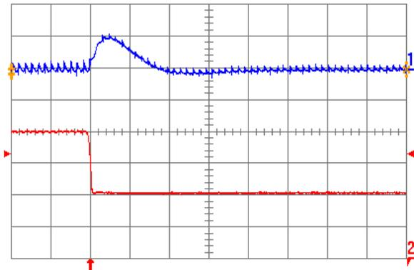
Fig. 1.5V.7: Output voltage response for  $V_{out} = 1.5\text{ V}$  to negative load current step change from 20 A to 10 A with slew rate of  $-5\text{ A}/\mu\text{s}$  at  $V_{in} = 12\text{ V}$ . Top trace: output voltage (200 mV/div.); Bottom trace: load current (5 A/div.).  $C_o = 100\text{ }\mu\text{F}$  ceramic. Time scale: 20  $\mu\text{s}$ /div.
