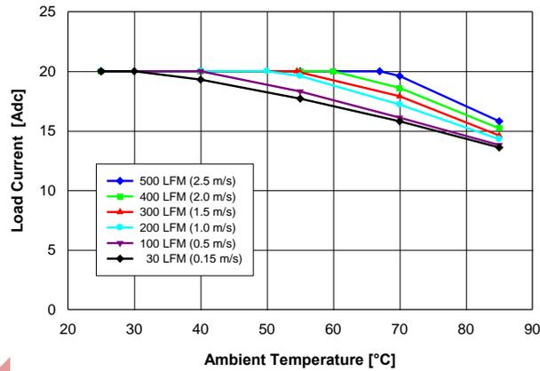
Fig. 3.3V.1: Available load current vs. ambient temperature and airflow rates for  $V_{out} = 3.3\text{ V}$  converter mounted vertically with  $V_{in} = 12\text{ V}$ , and maximum MOSFET temperature  $\leq 120\text{ }^\circ\text{C}$ .
