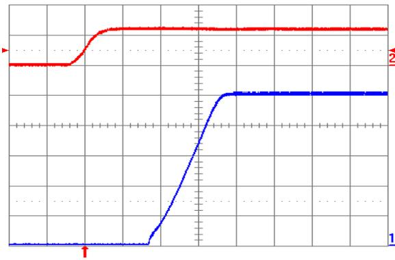
Fig. 5.0V.4: Turn-on transient for  $V_{out} = 5.0\text{ V}$  with application of  $V_{in}$  at full rated load current (resistive) and  $100\text{ }\mu\text{F}$  external capacitance at  $V_{in} = 12\text{ V}$ . Top trace:  $V_{in}$  (10 V/div.); Bottom trace: output voltage (1 V/div.); Time scale: 2 ms/div.
