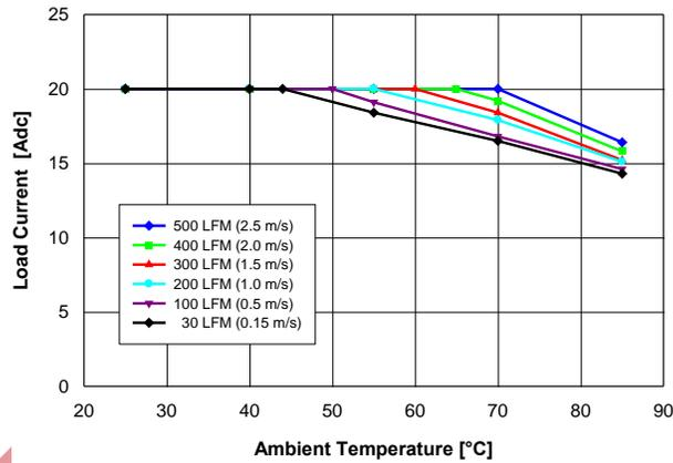
Fig. 1.0V.1: Available load current vs. ambient temperature and airflow rates for  $V_{out} = 1.0\text{ V}$  converter mounted vertically with  $V_{in} = 12\text{ V}$ , and maximum MOSFET temperature  $\leq 120\text{ }^\circ\text{C}$ .
