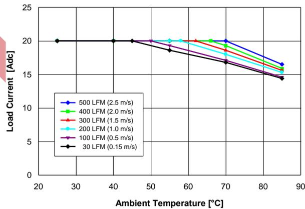
Fig. 0.7525V.1: Available load current vs. ambient temperature and airflow rates for  $V_{out} = 1.0\text{ V}$  converter mounted vertically with  $V_{in} = 12\text{ V}$ , and maximum MOSFET temperature  $\leq 120\text{ }^\circ\text{C}$ .
