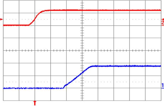
Fig. 1.8V.4: Turn-on transient for  $V_{out} = 1.8\text{ V}$  with application of  $V_{in}$  at full rated load current (resistive) and  $100\ \mu\text{F}$  external capacitance at  $V_{in} = 12\text{ V}$ . Top trace:  $V_{in}$  ( $10\text{ V/div.}$ ); Bottom trace: output voltage ( $1\text{ V/div.}$ ); Time scale:  $2\text{ ms/div.}$
