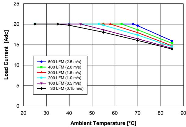
Fig. 2.0V.1: Available load current vs. ambient temperature and airflow rates for  $V_{out} = 2.0\text{ V}$  converter mounted vertically with  $V_{in} = 12\text{ V}$ , and maximum MOSFET temperature  $\leq 120\text{ }^{\circ}\text{C}$ .
