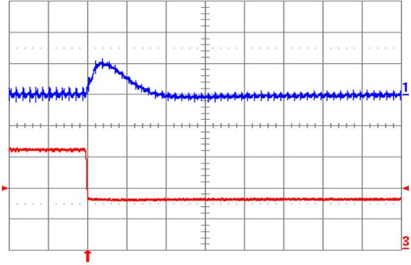
Fig. 2.0V.7: Output voltage response for  $V_{out} = 2.0\text{ V}$  to negative load current step change from 20 A to 10 A with slew rate of  $-5\text{ A}/\mu\text{s}$  at  $V_{in} = 12\text{ V}$ . Top trace: output voltage (200 mV/div.); Bottom trace: load current (5 A/div.).  $C_o = 100\ \mu\text{F}$  ceramic. Time scale:  $20\ \mu\text{s}/\text{div}$ .
