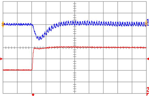
Fig. 3.3V.6: Output voltage response for  $V_{out} = 3.3\text{ V}$  to positive load current step change from  $10\text{ A}$  to  $20\text{ A}$  with slew rate of  $5\text{ A}/\mu\text{s}$  at  $V_{in} = 12\text{ V}$ . Top trace: output voltage ( $200\text{ mV/div.}$ ); Bottom trace: load current ( $5\text{ A/div.}$ ).  $C_o = 100\ \mu\text{F}$  ceramic. Time scale:  $20\ \mu\text{s/div.}$
