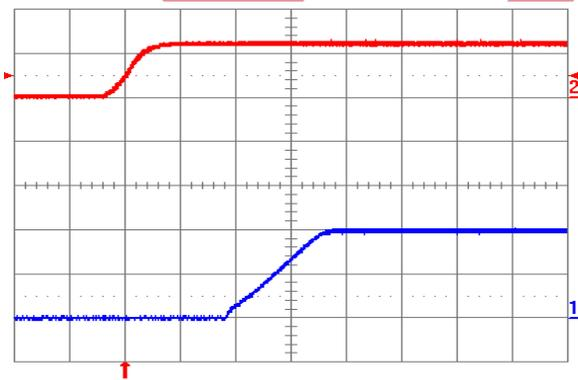
Fig. 2.0V.4: Turn-on transient for  $V_{out} = 2.0\text{ V}$  with application of  $V_{in}$  at full rated load current (resistive) and  $100\text{ }\mu\text{F}$  external capacitance at  $V_{in} = 12\text{ V}$ . Top trace:  $V_{in}$  (10 V/div.); Bottom trace: output voltage (1 V/div.); Time scale: 2 ms/div.
