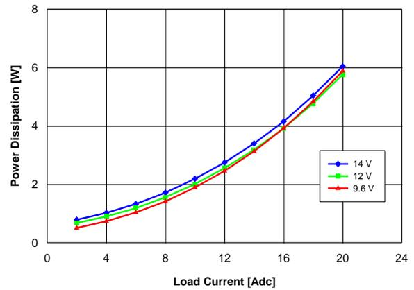
Fig. 2.0V.3: Power loss vs. load current and input voltage for  $V_{out} = 2.0\text{ V}$  converter mounted vertically with air flowing at a rate of 200 LFM (1 m/s) and  $T_a = 25\text{ }^{\circ}\text{C}$ .
