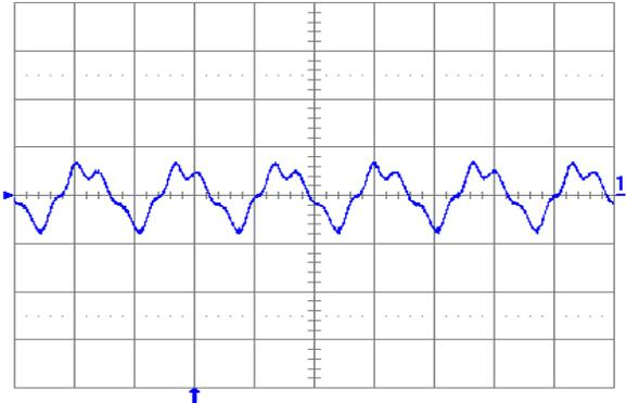
Fig. 3.3V.5: Output voltage ripple ( $20\text{ mV/div.}$ ) at full rated load current into a resistive load with external capacitance  $100\ \mu\text{F}$  ceramic +  $1\ \mu\text{F}$  ceramic and  $V_{in} = 12\text{ V}$  for  $V_{out} = 3.3\text{ V}$ . Time scale:  $2\ \mu\text{s/div.}$
