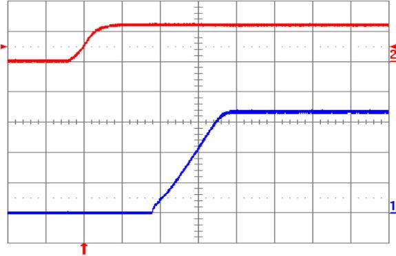
Fig. 3.3V.4: Turn-on transient for  $V_{out} = 3.3\text{ V}$  with application of  $V_{in}$  at full rated load current (resistive) and  $100\ \mu\text{F}$  external capacitance at  $V_{in} = 12\text{ V}$ . Top trace:  $V_{in}$  ( $10\text{ V/div.}$ ); Bottom trace: output voltage ( $1\text{ V/div.}$ ); Time scale:  $2\text{ ms/div.}$
