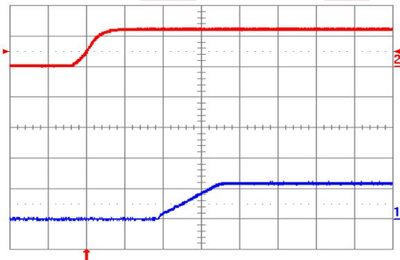
Fig. 1.2V.4: Turn-on transient for  $V_{out} = 1.2\text{ V}$  with application of  $V_{in}$  at full rated load current (resistive) and  $100\text{ }\mu\text{F}$  external capacitance at  $V_{in} = 12\text{ V}$ . Top trace:  $V_{in}$  (10 V/div.); Bottom trace: output voltage (1 V/div.); Time scale: 2 ms/div.
