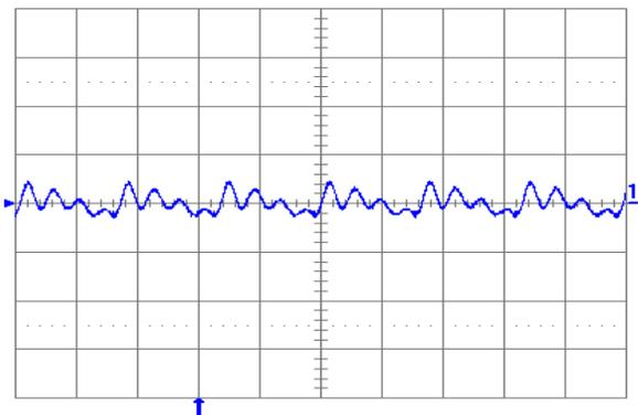
Fig. 1.2V.5: Output voltage ripple (20 mV/div.) at full rated load current into a resistive load with external capacitance  $100\text{ }\mu\text{F}$  ceramic +  $1\text{ }\mu\text{F}$  ceramic and  $V_{in} = 12\text{ V}$  for  $V_{out} = 1.2\text{ V}$ . Time scale: 2  $\mu\text{s}$ /div.
