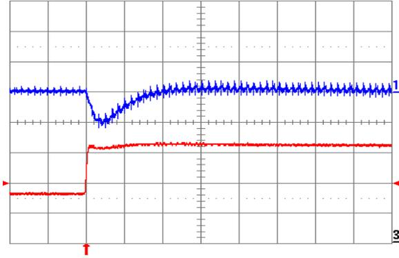
Fig. 2.0V.6: Output voltage response for  $V_{out} = 2.0\text{ V}$  to positive load current step change from 10 A to 20 A with slew rate of  $5\text{ A}/\mu\text{s}$  at  $V_{in} = 12\text{ V}$ . Top trace: output voltage (200 mV/div.); Bottom trace: load current (5 A/div.).  $C_o = 100\ \mu\text{F}$  ceramic. Time scale:  $20\ \mu\text{s}/\text{div}$ .
