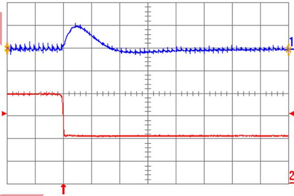
Fig. 1.0V.7: Output voltage response for  $V_{out} = 1.0\text{ V}$  to negative load current step change from 20 A to 10 A with slew rate of  $-5\text{ A}/\mu\text{s}$  at  $V_{in} = 12\text{ V}$ . Top trace: output voltage (200 mV/div.); Bottom trace: load current (5 A/div.).  $C_o = 100\ \mu\text{F}$  ceramic. Time scale: 20  $\mu\text{s}$ /div.
