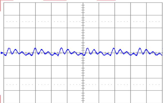
Fig. 0.7525V.5: Output voltage ripple (20 mV/div.) at full rated load current into a resistive load with external capacitance  $100 \mu F$  ceramic +  $1 \mu F$  ceramic and  $V_{in} = 12 V$  for  $V_{out} = 0.7525V$ . Time scale: 2  $\mu s$ /div.
