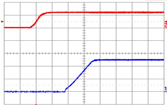
Fig. 2.5V.4: Turn-on transient for  $V_{out} = 2.5$  V with application of  $V_{in}$  at full rated load current (resistive) and 100  $\mu$ F external capacitance at  $V_{in} = 12$  V. Top trace:  $V_{in}$  (10 V/div.); Bottom trace: output voltage (1 V/div.); Time scale: 2 ms/div.
