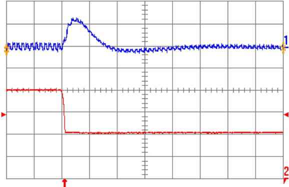
Fig. 5.0V.7: Output voltage response for  $V_{out} = 5.0\text{ V}$  to negative load current step change from 20 A to 10 A with slew rate of  $-5\text{ A}/\mu\text{s}$  at  $V_{in} = 12\text{ V}$ . Top trace: output voltage (200 mV/div.); Bottom trace: load current (5 A/div.).  $C_o = 100\text{ }\mu\text{F}$  ceramic. Time scale:  $20\text{ }\mu\text{s}/\text{div}$ .
