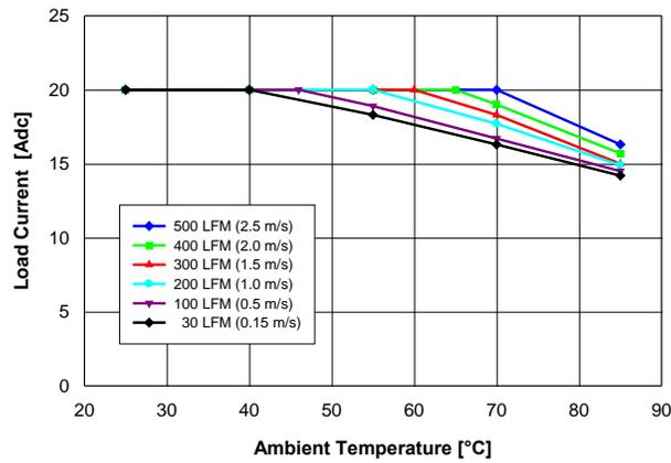
Fig. 1.8V.1: Available load current vs. ambient temperature and airflow rates for  $V_{out} = 1.8\text{ V}$  converter mounted vertically with  $V_{in} = 12\text{ V}$ , and maximum MOSFET temperature  $\leq 120\text{ }^\circ\text{C}$ .
