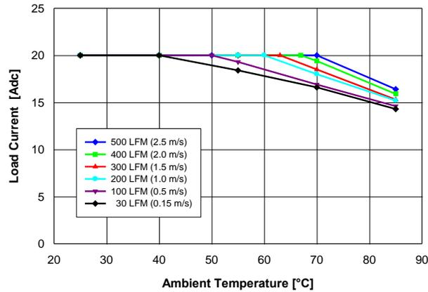
Fig. 1.2V.1: Available load current vs. ambient temperature and airflow rates for  $V_{out} = 1.2\text{ V}$  converter mounted vertically with  $V_{in} = 12\text{ V}$ , and maximum MOSFET temperature  $\leq 120\text{ }^{\circ}\text{C}$ .
