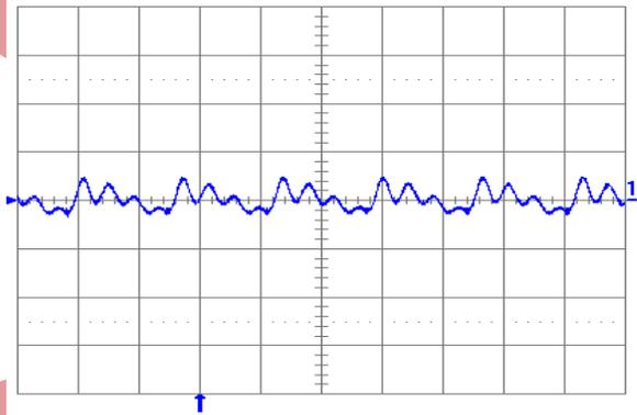
Fig. 1.5V.5: Output voltage ripple (20 mV/div.) at full rated load current into a resistive load with external capacitance  $100\text{ }\mu\text{F}$  ceramic +  $1\text{ }\mu\text{F}$  ceramic and  $V_{in} = 12\text{ V}$  for  $V_{out} = 1.5\text{ V}$ . Time scale: 2  $\mu\text{s}$ /div.
