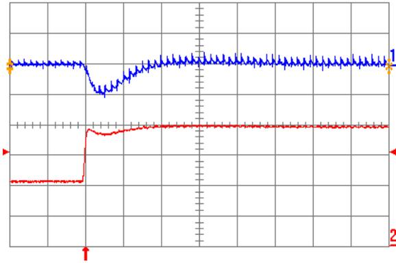
Fig. 1.2V.6: Output voltage response for  $V_{out} = 1.2\text{ V}$  to positive load current step change from 10 A to 20 A with slew rate of  $5\text{ A}/\mu\text{s}$  at  $V_{in} = 12\text{ V}$ . Top trace: output voltage (200 mV/div.); Bottom trace: load current (5 A/div.).  $C_o = 100\ \mu\text{F}$  ceramic. Time scale:  $20\ \mu\text{s}/\text{div}$ .
