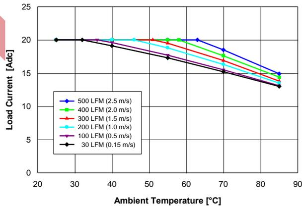
Fig. 2.5V.1: Available load current vs. ambient temperature and airflow rates for  $V_{out} = 2.5\text{ V}$  converter mounted vertically with  $V_{in} = 12\text{ V}$ , and maximum MOSFET temperature  $\leq 120\text{ }^\circ\text{C}$ .
