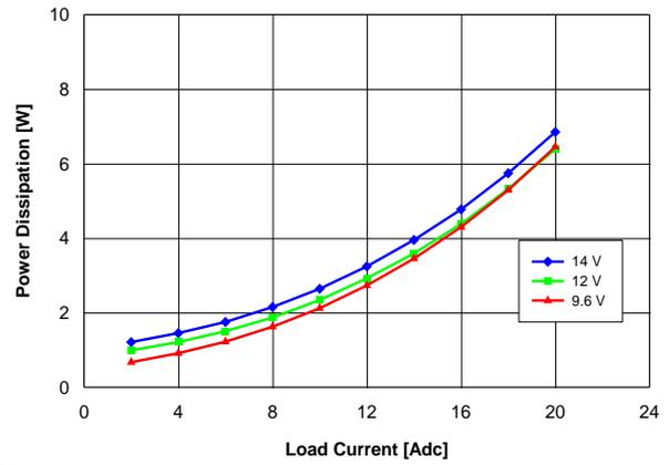
Fig. 5.0V.3: Power loss vs. load current and input voltage for  $V_{out} = 5.0\text{ V}$  converter mounted vertically with air flowing at a rate of 200 LFM (1 m/s) and  $T_a = 25\text{ }^{\circ}\text{C}$ .
