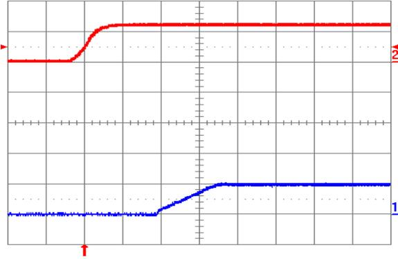
Fig. 1.0V.4: Turn-on transient for  $V_{out} = 1.0\text{ V}$  with application of  $V_{in}$  at full rated load current (resistive) and  $100\ \mu\text{F}$  external capacitance at  $V_{in} = 12\text{ V}$ . Top trace:  $V_{in}$  (10 V/div.); Bottom trace: output voltage (1 V/div.); Time scale: 2 ms/div.
