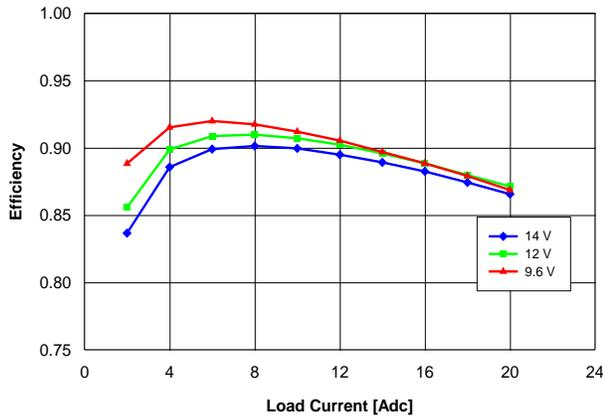
Fig. 2.0V.2: Efficiency vs. load current and input voltage for  $V_{out} = 2.0\text{ V}$  converter mounted vertically with air flowing at a rate of 200 LFM (1 m/s) and  $T_a = 25\text{ }^{\circ}\text{C}$ .
