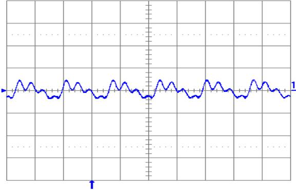
Fig. 1.8V.5: Output voltage ripple ( $20\text{ mV/div.}$ ) at full rated load current into a resistive load with external capacitance  $100\ \mu\text{F}$  ceramic +  $1\ \mu\text{F}$  ceramic and  $V_{in} = 12\text{ V}$  for  $V_{out} = 1.8\text{ V}$ . Time scale:  $2\ \mu\text{s/div.}$
