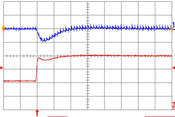
Fig. 1.0V.6: Output voltage response for  $V_{out} = 1.0\text{ V}$  to positive load current step change from 10 A to 20 A with slew rate of  $5\text{ A}/\mu\text{s}$  at  $V_{in} = 12\text{ V}$ . Top trace: output voltage (200 mV/div.); Bottom trace: load current (5 A/div.).  $C_o = 100\ \mu\text{F}$  ceramic. Time scale: 20  $\mu\text{s}$ /div.
