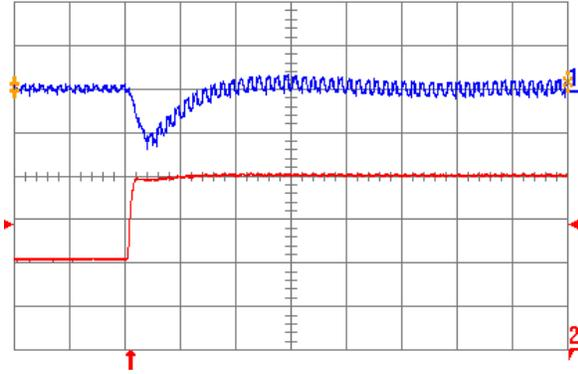
Fig. 5.0V.6: Output voltage response for  $V_{out} = 5.0\text{ V}$  to positive load current step change from 10 A to 20 A with slew rate of  $5\text{ A}/\mu\text{s}$  at  $V_{in} = 12\text{ V}$ . Top trace: output voltage (200 mV/div.); Bottom trace: load current (5 A/div.).  $C_o = 100\text{ }\mu\text{F}$  ceramic. Time scale:  $20\text{ }\mu\text{s}/\text{div}$ .
