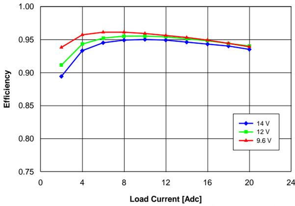
Fig. 5.0V.2: Efficiency vs. load current and input voltage for  $V_{out} = 5.0\text{ V}$  converter mounted vertically with air flowing at a rate of 200 LFM (1 m/s) and  $T_a = 25\text{ }^{\circ}\text{C}$ .
