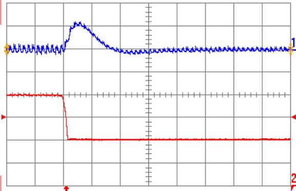
Fig. 3.3V.7: Output voltage response for  $V_{out} = 3.3\text{ V}$  to negative load current step change from  $20\text{ A}$  to  $10\text{ A}$  with slew rate of  $-5\text{ A}/\mu\text{s}$  at  $V_{in} = 12\text{ V}$ . Top trace: output voltage ( $200\text{ mV/div.}$ ); Bottom trace: load current ( $5\text{ A/div.}$ ).  $C_o = 100\ \mu\text{F}$  ceramic. Time scale:  $20\ \mu\text{s/div.}$
