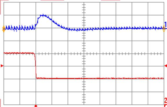
Fig. 1.8V.7: Output voltage response for  $V_{out} = 1.8\text{ V}$  to negative load current step change from  $20\text{ A}$  to  $10\text{ A}$  with slew rate of  $-5\text{ A}/\mu\text{s}$  at  $V_{in} = 12\text{ V}$ . Top trace: output voltage ( $200\text{ mV/div.}$ ); Bottom trace: load current ( $5\text{ A/div.}$ ).  $C_o = 100\ \mu\text{F}$  ceramic. Time scale:  $20\ \mu\text{s/div.}$
