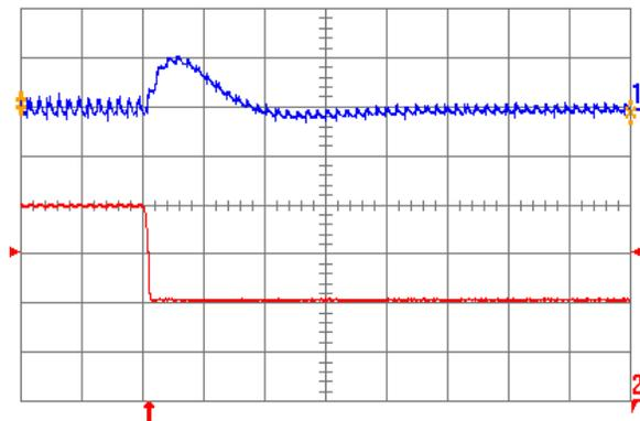
Fig. 2.5V.7: Output voltage response for  $V_{out} = 2.5$  V to negative load current step change from 20 A to 10 A with slew rate of -5A/ $\mu$ s at  $V_{in} = 12$  V. Top trace: output voltage (200 mV/div.); Bottom trace: load current (5 A/div.).  $C_o = 100$   $\mu$ F ceramic. Time scale: 20  $\mu$ s/div.
