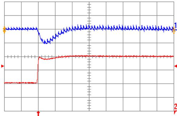
Fig. 1.5V.6: Output voltage response for  $V_{out} = 1.5\text{ V}$  to positive load current step change from 10 A to 20 A with slew rate of  $5\text{ A}/\mu\text{s}$  at  $V_{in} = 12\text{ V}$ . Top trace: output voltage (200 mV/div.); Bottom trace: load current (5 A/div.).  $C_o = 100\text{ }\mu\text{F}$  ceramic. Time scale: 20  $\mu\text{s}$ /div.
