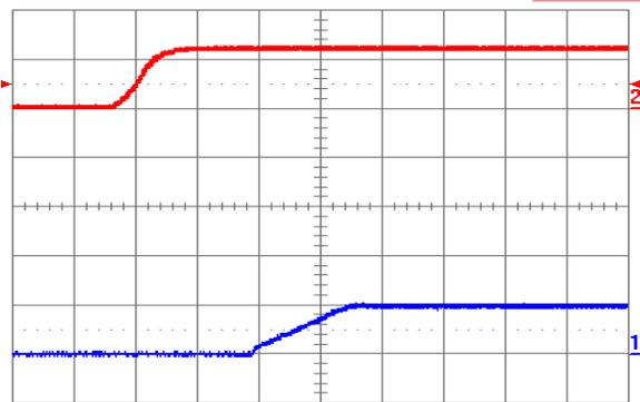
Fig. 0.7525V.4: Turn-on transient for  $V_{out} = 0.7525 V$  with application of  $V_{in}$  at full rated load current (resistive) and  $100 \mu F$  external capacitance at  $V_{in} = 12 V$ . Top trace:  $V_{in}$  (10 V/div.); Bottom trace: output voltage (1 V/div.); Time scale: 2 ms/div.
