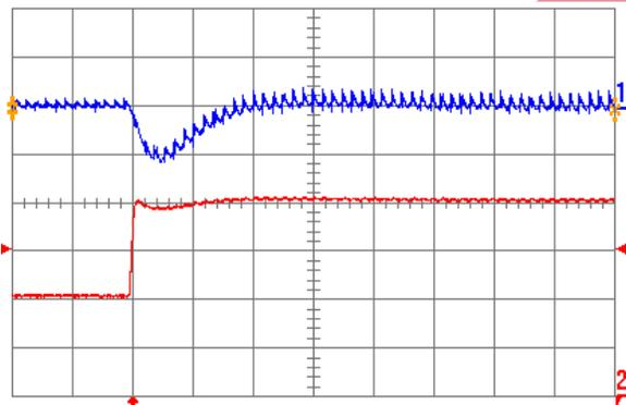
Fig. 1.8V.6: Output voltage response for  $V_{out} = 1.8\text{ V}$  to positive load current step change from  $10\text{ A}$  to  $20\text{ A}$  with slew rate of  $5\text{ A}/\mu\text{s}$  at  $V_{in} = 12\text{ V}$ . Top trace: output voltage ( $200\text{ mV/div.}$ ); Bottom trace: load current ( $5\text{ A/div.}$ ).  $C_o = 100\ \mu\text{F}$  ceramic. Time scale:  $20\ \mu\text{s/div.}$
