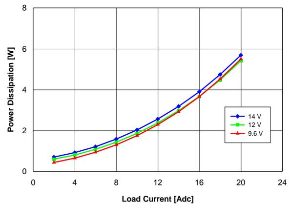
Fig. 1.2V.3: Power loss vs. load current and input voltage for  $V_{out} = 1.2\text{ V}$  converter mounted vertically with air flowing at a rate of 200 LFM (1 m/s) and  $T_a = 25\text{ }^{\circ}\text{C}$ .
