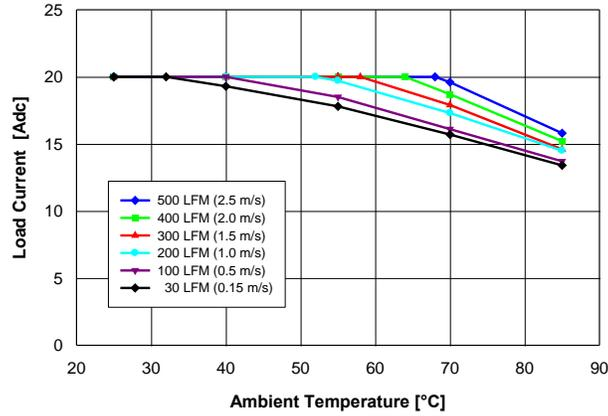
Fig. 5.0V.1: Available load current vs. ambient temperature and airflow rates for  $V_{out} = 5.0\text{ V}$  converter mounted vertically with  $V_{in} = 12\text{ V}$ , and maximum MOSFET temperature  $\leq 120\text{ }^{\circ}\text{C}$ .
