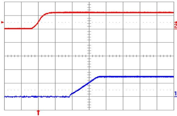
Fig. 1.5V.4: Turn-on transient for  $V_{out} = 1.5\text{ V}$  with application of  $V_{in}$  at full rated load current (resistive) and  $100\text{ }\mu\text{F}$  external capacitance at  $V_{in} = 12\text{ V}$ . Top trace:  $V_{in}$  (10 V/div.); Bottom trace: output voltage (1 V/div.); Time scale: 2 ms/div.
