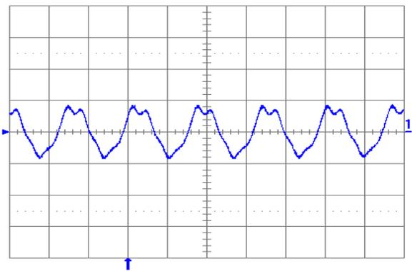
Fig. 5.0V.5: Output voltage ripple (20 mV/div.) at full rated load current into a resistive load with external capacitance  $100\text{ }\mu\text{F}$  ceramic +  $1\text{ }\mu\text{F}$  ceramic and  $V_{in} = 12\text{ V}$  for  $V_{out} = 5.0\text{ V}$ . Time scale: 2  $\mu\text{s}$ /div.
