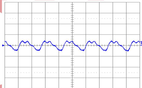
Fig. 2.5V.5: Output voltage ripple (20 mV/div.) at full rated load current into a resistive load with external capacitance 100  $\mu$ F ceramic + 1  $\mu$ F ceramic and  $V_{in} = 12$  V for  $V_{out} = 2.5$  V. Time scale: 2  $\mu$ s/div.
