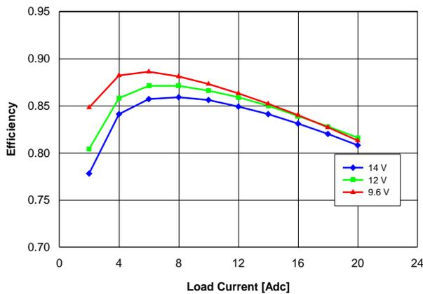
Fig. 1.2V.2: Efficiency vs. load current and input voltage for  $V_{out} = 1.2\text{ V}$  converter mounted vertically with air flowing at a rate of 200 LFM (1 m/s) and  $T_a = 25\text{ }^{\circ}\text{C}$ .
