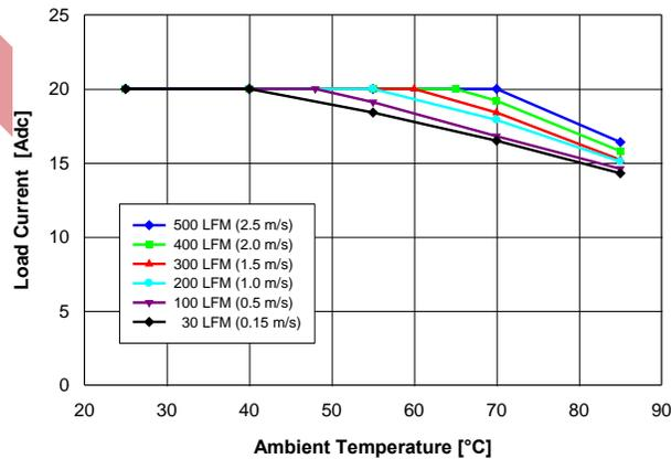
Fig. 1.5V.1: Available load current vs. ambient temperature and airflow rates for  $V_{out} = 1.5\text{ V}$  converter mounted vertically with  $V_{in} = 12\text{ V}$ , air flowing and maximum MOSFET temperature  $\leq 120\text{ }^\circ\text{C}$ .
