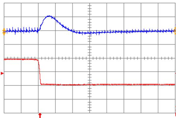
Fig. 0.7525V.7: Output voltage response for  $V_{out} = 0.7525 V$  to negative load current step change from 20 A to 10 A with slew rate of  $-5 A/\mu s$  at  $V_{in} = 12 V$ . Top trace: output voltage (200 mV/div.); Bottom trace: load current (5 A/div.).  $C_o = 100 \mu F$  ceramic. Time scale: 20  $\mu s$ /div.
