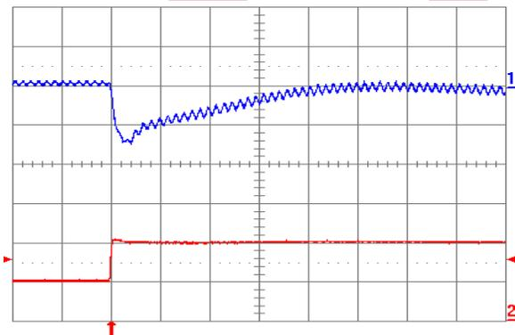
Fig. 2.0V.7: Output voltage response for  $V_{out} = 2.0\text{ V}$  to positive load current step change from 10 A to 20 A with slew rate of  $5\text{ A}/\mu\text{s}$  at  $V_{in} = 5\text{ V}$ . Top trace: output voltage (100 mV/div.); Bottom trace: load current (10 A/div.).  $C_o = 100\text{ }\mu\text{F}$  ceramic. Time scale: 20  $\mu\text{s}$ /div.
