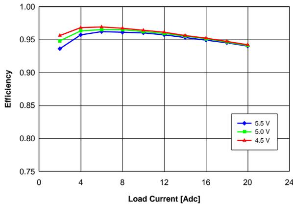
Fig. 3.3V.3: Efficiency vs. load current and input voltage for  $V_{out} = 3.3\text{ V}$  converter mounted vertically with air flowing from pin 1 and pin 6 to pins 2 - 5 at a rate of 200 LFM (1 m/s) and  $T_a = 25\text{ }^{\circ}\text{C}$ .
