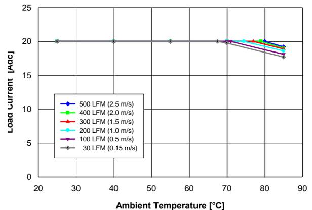
Fig. 1.2V.2: Available load current vs. ambient temperature and airflow rates for  $V_{out} = 1.2\text{ V}$  converter mounted horizontally with  $V_{in} = 5\text{ V}$ , air flowing from pin 1 and pin 6 to pins 2 – 5, and maximum MOSFET temperature  $\leq 120\text{ }^\circ\text{C}$ .
