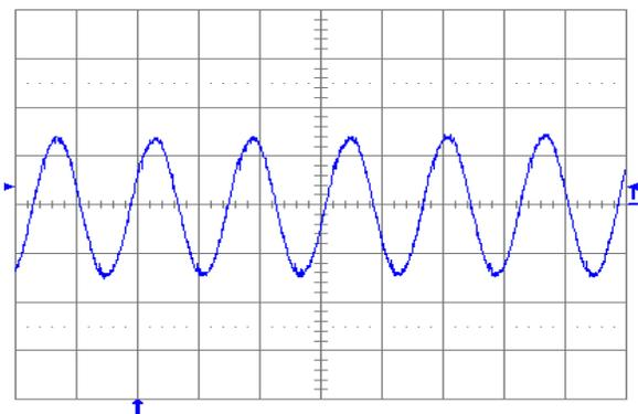
Fig. 1.8V.6: Output voltage ripple (20 mV/div.) at full rated load current into a resistive load with external capacitance  $100\ \mu\text{F}$  ceramic +  $1\ \mu\text{F}$  ceramic and  $V_{in} = 5\text{ V}$  for  $V_{out} = 1.8\text{ V}$ . Time scale: 2 μs/div.
