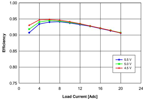
Fig. 2.0V.3: Efficiency vs. load current and input voltage for  $V_{out} = 2.0\text{ V}$  converter mounted vertically with air flowing from pin 1 and pin 6 to pins 2 – 5 at a rate of 200 LFM (1 m/s) and  $T_a = 25\text{ }^\circ\text{C}$ .
