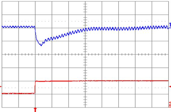
Fig. 2.5V.7: Output voltage response for  $V_{out} = 2.5\text{ V}$  to positive load current step change from 10 A to 20 A with slew rate of  $5\text{ A}/\mu\text{s}$  at  $V_{in} = 5\text{ V}$ . Top trace: output voltage (100 mV/div.); Bottom trace: load current (10 A/div.).  $C_o = 100\ \mu\text{F}$  ceramic. Time scale: 20  $\mu\text{s}$ /div.
