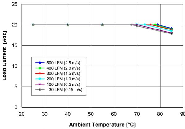
Fig. 1.5V.1: Available load current vs. ambient temperature and airflow rates for  $V_{out} = 1.5\text{ V}$  converter mounted vertically with  $V_{in} = 5\text{ V}$ , air flowing from pin 1 and pin 6 to pins 2 – 5, and maximum MOSFET temperature  $\leq 120^\circ\text{C}$ .
