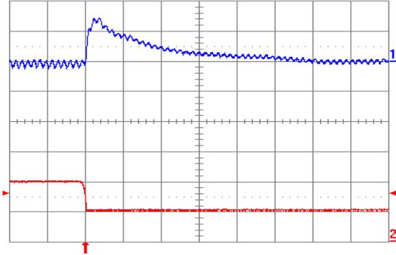
Fig. 3.3V.8: Output voltage response for  $V_{out} = 3.3\text{ V}$  to negative load current step change from 20 A to 10 A with slew rate of  $-5\text{ A}/\mu\text{s}$  at  $V_{in} = 5\text{ V}$ . Top trace: output voltage (100 mV/div.); Bottom trace: load current (10 A/div.).  $C_o = 100\text{ }\mu\text{F}$  ceramic. Time scale:  $20\text{ }\mu\text{s}/\text{div}$ .
