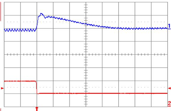
Fig. 0.7525V.8: Output voltage response for  $V_{out} = 0.7525$  V to negative load current step change from 20 A to 10 A with slew rate of  $-5 \text{ A}/\mu\text{s}$  at  $V_{in} = 5$  V. Top trace: output voltage (100 mV/div.); Bottom trace: load current (10 A/div.).  $C_o = 100 \mu\text{F}$  ceramic. Time scale: 20  $\mu\text{s}$ /div.
