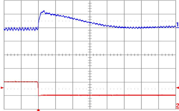
Fig. 1.8V.8: Output voltage response for  $V_{out} = 1.8\text{ V}$  to negative load current step change from 20 A to 10 A with slew rate of  $-5\text{ A}/\mu\text{s}$  at  $V_{in} = 5\text{ V}$ . Top trace: output voltage (100 mV/div.); Bottom trace: load current (10 A/div.).  $C_o = 100\text{ }\mu\text{F}$  ceramic. Time scale:  $20\text{ }\mu\text{s}/\text{div}$ .
