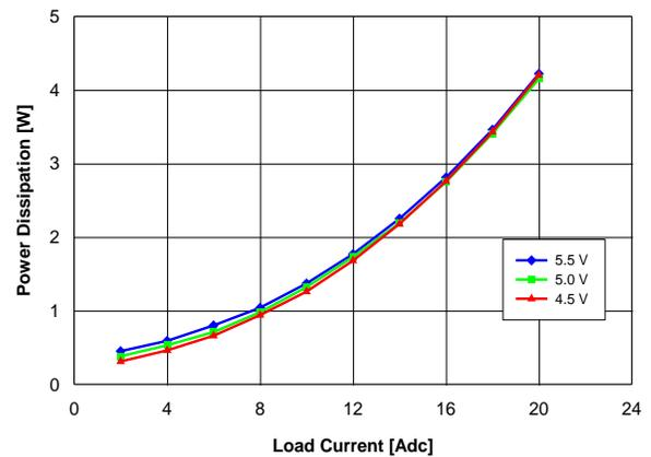
Fig. 2.5V.4: Power loss vs. load current and input voltage for  $V_{out} = 2.5\text{ V}$  converter mounted vertically with air flowing from pin 1 and pin 6 to pins 2 – 5 at a rate of 200 LFM (1 m/s) and  $T_a = 25\text{ }^\circ\text{C}$ .
