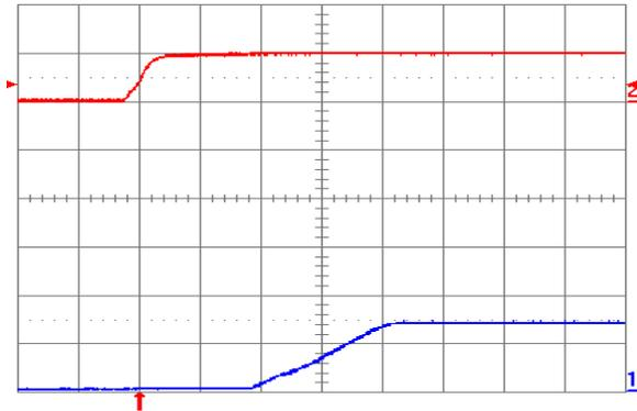
Fig. 0.7525V.5: Turn-on transient for  $V_{out} = 0.7525$  V with application of  $V_{in}$  at full rated load current (resistive) and  $100 \mu\text{F}$  external capacitance at  $V_{in} = 5$  V. Top trace:  $V_{in}$  (5 V/div.); Bottom trace: output voltage (1 V/div.); Time scale: 2 ms/div.
