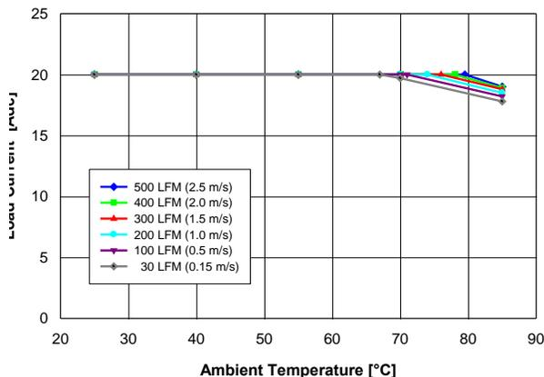
Fig. 2.0V.1: Available load current vs. ambient temperature and airflow rates for  $V_{out} = 2.0\text{ V}$  converter mounted vertically with  $V_{in} = 5\text{ V}$ , air flowing from pin 1 and pin 6 to pins 2 – 5, and maximum MOSFET temperature  $\leq 120\text{ }^\circ\text{C}$ .
