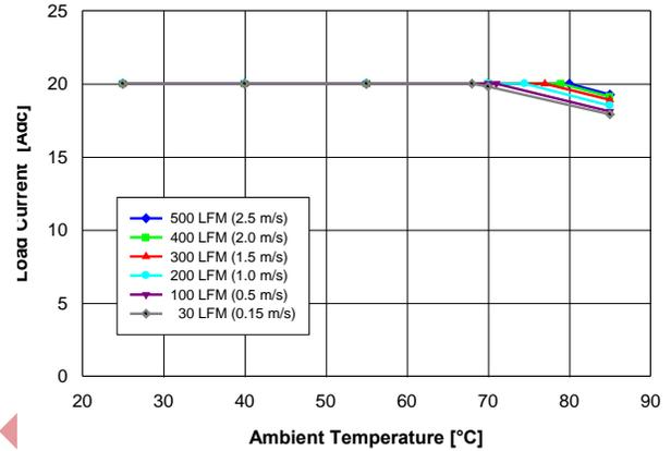
Fig. 1.0V.2: Available load current vs. ambient temperature and airflow rates for  $V_{out} = 1.0\text{ V}$  converter mounted horizontally with  $V_{in} = 5\text{ V}$ , air flowing from pin 1 and pin 6 to pins 2 - 5, and maximum MOSFET temperature  $\leq 120\text{ }^{\circ}\text{C}$ .
