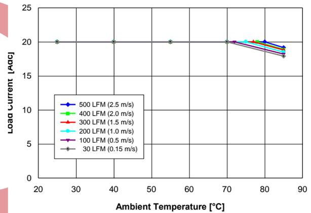
Fig. 0.7525V.2: Available load current vs. ambient temperature and airflow rates for  $V_{out} = 0.7525\text{ V}$  converter mounted horizontally with  $V_{in} = 5\text{ V}$ , air flowing from pin 1 and pin 6 to pins 2 – 5, and maximum MOSFET temperature  $\leq 120\text{ }^\circ\text{C}$ .
