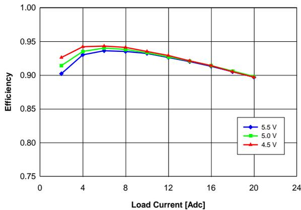
Fig. 1.8V.3: Efficiency vs. load current and input voltage for  $V_{out} = 1.8\text{ V}$  converter mounted vertically with air flowing from pin 1 and pin 6 to pins 2 - 5 at a rate of 200 LFM (1 m/s) and  $T_a = 25^\circ\text{C}$ .
