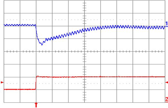
Fig. 1.8V.7: Output voltage response for  $V_{out} = 1.8\text{ V}$  to positive load current step change from 10 A to 20 A with slew rate of  $5\text{ A}/\mu\text{s}$  at  $V_{in} = 5\text{ V}$ . Top trace: output voltage (100 mV/div.); Bottom trace: load current (10 A/div.).  $C_o = 100\text{ }\mu\text{F}$  ceramic. Time scale:  $20\text{ }\mu\text{s}/\text{div}$ .
