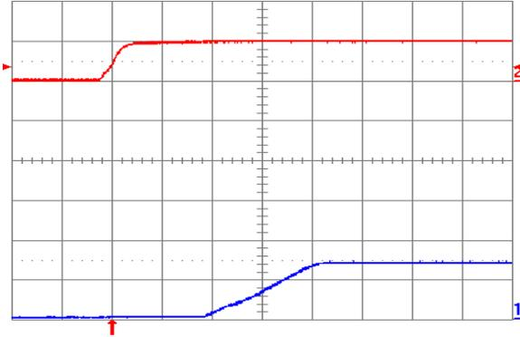
Fig. 1.5V.5: Turn-on transient for  $V_{out} = 1.5\text{ V}$  with application of  $V_{in}$  at full rated load current (resistive) and  $100\ \mu\text{F}$  external capacitance at  $V_{in} = 5\text{ V}$ . Top trace:  $V_{in}$  (5 V/div.); Bottom trace: output voltage (1 V/div.); Time scale: 2 ms/div.
