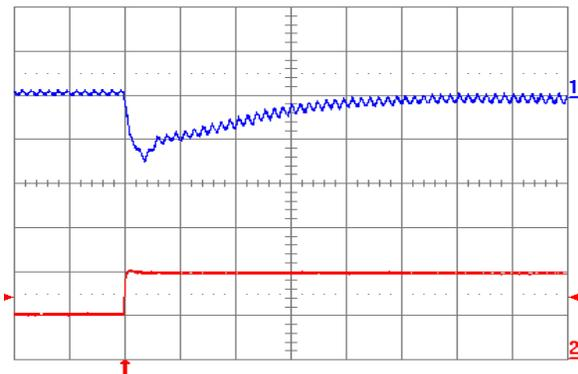
Fig. 1.2V.7: Output voltage response for  $V_{out} = 1.2\text{ V}$  to positive load current step change from 10 A to 20 A with slew rate of  $5\text{ A}/\mu\text{s}$  at  $V_{in} = 5\text{ V}$ . Top trace: output voltage (100 mV/div.); Bottom trace: load current (10 A/div.).  $C_o = 100\text{ }\mu\text{F}$  ceramic. Time scale: 20  $\mu\text{s}$ /div.
