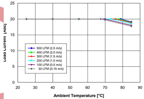
Fig. 1.5V.2: Available load current vs. ambient temperature and airflow rates for  $V_{out} = 1.5\text{ V}$  converter mounted horizontally with  $V_{in} = 5\text{ V}$ , air flowing from pin 1 and pin 6 to pins 2 – 5, and maximum MOSFET temperature  $\leq 120^\circ\text{C}$ .
