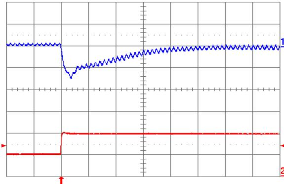
Fig. 1.5V.7: Output voltage response for  $V_{out} = 1.5\text{ V}$  to positive load current step change from 10 A to 20 A with slew rate of  $5\text{ A}/\mu\text{s}$  at  $V_{in} = 5\text{ V}$ . Top trace: output voltage (100 mV/div.); Bottom trace: load current (10 A/div.).  $C_o = 100\ \mu\text{F}$  ceramic. Time scale: 20  $\mu\text{s}$ /div.
