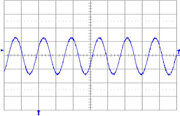
Fig. 2.5V.6: Output voltage ripple (20 mV/div.) at full rated load current into a resistive load with external capacitance  $100\ \mu\text{F}$  ceramic +  $1\ \mu\text{F}$  ceramic and  $V_{in} = 5\text{ V}$  for  $V_{out} = 2.5\text{ V}$ . Time scale: 2  $\mu\text{s}$ /div.
