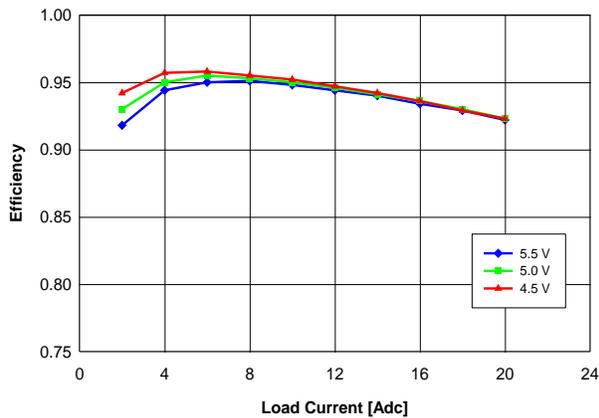
Fig. 2.5V.3: Efficiency vs. load current and input voltage for  $V_{out} = 2.5\text{ V}$  converter mounted vertically with air flowing from pin 1 and pin 6 to pins 2 – 5 at a rate of 200 LFM (1 m/s) and  $T_a = 25\text{ }^\circ\text{C}$ .
