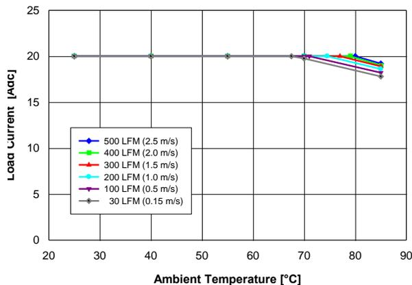
Fig. 1.2V.1: Available load current vs. ambient temperature and airflow rates for  $V_{out} = 1.2\text{ V}$  converter mounted vertically with  $V_{in} = 5\text{ V}$ , air flowing from pin 1 and pin 6 to pins 2 – 5, and maximum MOSFET temperature  $\leq 120\text{ }^\circ\text{C}$ .
