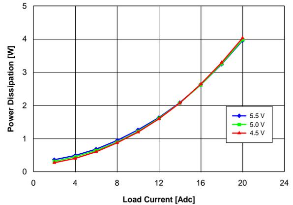
Fig. 1.2V.4: Power loss vs. load current and input voltage for  $V_{out} = 1.2\text{ V}$  converter mounted vertically with air flowing from pin 1 and pin 6 to pins 2 – 5 at a rate of 200 LFM (1 m/s) and  $T_a = 25\text{ }^\circ\text{C}$ .
