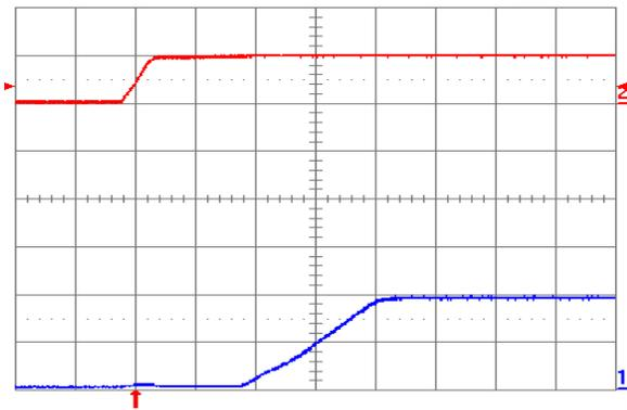
Fig. 2.0V.5: Turn-on transient for  $V_{out} = 2.0\text{ V}$  with application of  $V_{in}$  at full rated load current (resistive) and  $100\text{ }\mu\text{F}$  external capacitance at  $V_{in} = 5\text{ V}$ . Top trace:  $V_{in}$  (5 V/div.); Bottom trace: output voltage (1 V/div.); Time scale: 2 ms/div.
