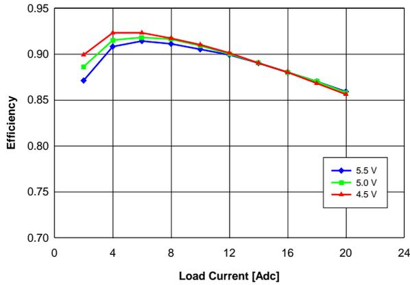
Fig. 1.2V.3: Efficiency vs. load current and input voltage for  $V_{out} = 1.2\text{ V}$  converter mounted vertically with air flowing from pin 1 and pin 6 to pins 2 – 5 at a rate of 200 LFM (1 m/s) and  $T_a = 25\text{ }^\circ\text{C}$ .
