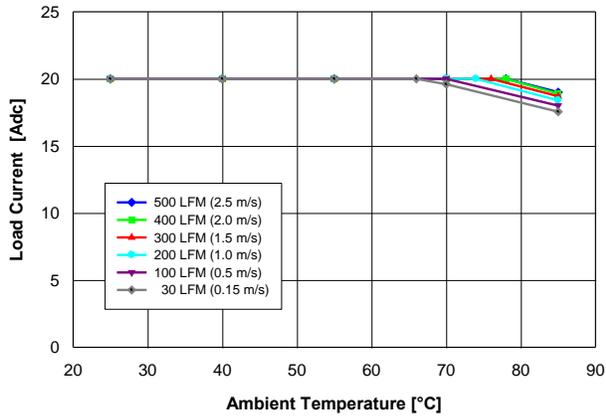
Fig. 3.3V.1: Available load current vs. ambient temperature and airflow rates for  $V_{out} = 3.3\text{ V}$  converter mounted vertically with  $V_{in} = 5\text{ V}$ , air flowing from pin 1 and pin 6 to pins 2 - 5, and maximum MOSFET temperature  $\leq 120\text{ }^{\circ}\text{C}$ .
