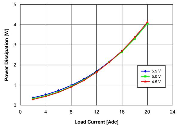
Fig. 1.5V.4: Power loss vs. load current and input voltage for  $V_{out} = 1.5\text{ V}$  converter mounted vertically with air flowing from pin 1 and pin 6 to pins 2 – 5 at a rate of 200 LFM (1 m/s) and  $T_a = 25^\circ\text{C}$ .
