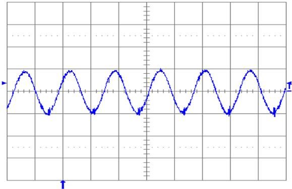
Fig. 0.7525V.6: Output voltage ripple (20 mV/div.) at full rated load current into a resistive load with external capacitance  $100 \mu\text{F}$  ceramic +  $1 \mu\text{F}$  ceramic and  $V_{in} = 5$  V for  $V_{out} = 0.7525$  V. Time scale: 2  $\mu\text{s}$ /div.
