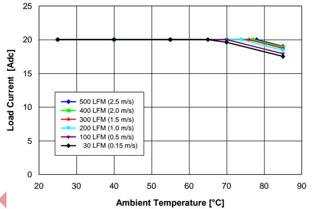
Fig. 3.3V.2: Available load current vs. ambient temperature and airflow rates for  $V_{out} = 3.3\text{ V}$  converter mounted horizontally with  $V_{in} = 5\text{ V}$ , air flowing from pin 1 and pin 6 to pins 2 - 5, and maximum MOSFET temperature  $\leq 120\text{ }^{\circ}\text{C}$ .
