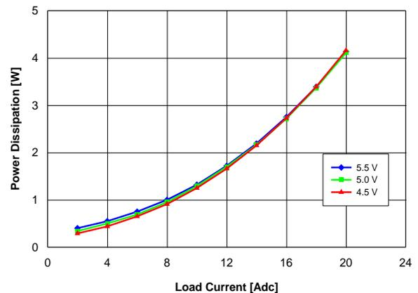
Fig. 1.8V.4: Power loss vs. load current and input voltage for  $V_{out} = 1.8\text{ V}$  converter mounted vertically with air flowing from pin 1 and pin 6 to pins 2 - 5 at a rate of 200 LFM (1 m/s) and  $T_a = 25^\circ\text{C}$ .
