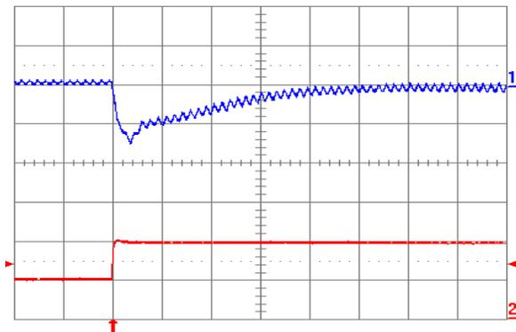
Fig. 0.7525V.7: Output voltage response for  $V_{out} = 0.7525$  V to positive load current step change from 10 A to 20 A with slew rate of  $5 \text{ A}/\mu\text{s}$  at  $V_{in} = 5$  V. Top trace: output voltage (100 mV/div.); Bottom trace: load current (10 A/div.).  $C_o = 100 \mu\text{F}$  ceramic. Time scale: 20  $\mu\text{s}$ /div.
