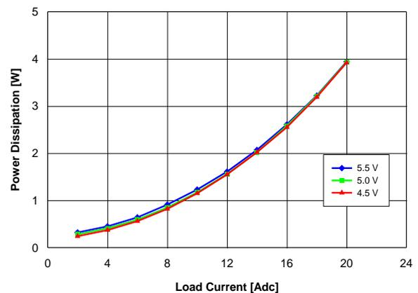
Fig. 0.7525V.4: Power loss vs. load current and input voltage for  $V_{out} = 0.7525\text{ V}$  converter mounted vertically with air flowing from pin 1 and pin 6 to pins 2 – 5 at a rate of 200 LFM (1 m/s) and  $T_a = 25\text{ }^\circ\text{C}$ .
