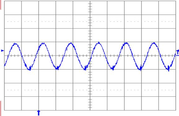
Fig. 1.2V.6: Output voltage ripple (20 mV/div.) at full rated load current into a resistive load with external capacitance  $100\text{ }\mu\text{F}$  ceramic +  $1\text{ }\mu\text{F}$  ceramic and  $V_{in} = 5\text{ V}$  for  $V_{out} = 1.2\text{ V}$ . Time scale: 2  $\mu\text{s}$ /div.
