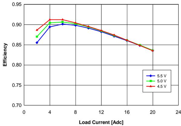
Fig. 1.0V.3: Efficiency vs. load current and input voltage for  $V_{out} = 1.0\text{ V}$  converter mounted vertically with air flowing from pin 1 and pin 6 to pins 2 - 5 at a rate of 200 LFM (1 m/s) and  $T_a = 25\text{ }^{\circ}\text{C}$ .
