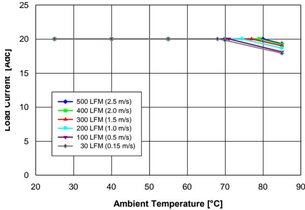
Fig. 1.0V.1: Available load current vs. ambient temperature and airflow rates for  $V_{out} = 1.0\text{ V}$  converter mounted vertically with  $V_{in} = 5\text{ V}$ , air flowing from pin 1 and pin 6 to pins 2 - 5, and maximum MOSFET temperature  $\leq 120\text{ }^{\circ}\text{C}$ .
