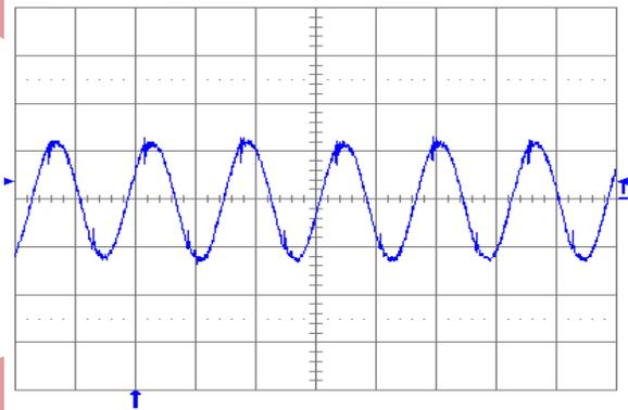
Fig. 2.0V.6: Output voltage ripple (20 mV/div.) at full rated load current into a resistive load with external capacitance  $100\text{ }\mu\text{F}$  ceramic +  $1\text{ }\mu\text{F}$  ceramic and  $V_{in} = 5\text{ V}$  for  $V_{out} = 2.0\text{ V}$ . Time scale: 2  $\mu\text{s}$ /div.
