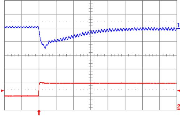
Fig. 1.0V.7: Output voltage response for  $V_{out} = 1.0\text{ V}$  to positive load current step change from 10 A to 20 A with slew rate of  $5\text{ A}/\mu\text{s}$  at  $V_{in} = 5\text{ V}$ . Top trace: output voltage (100 mV/div.); Bottom trace: load current (10 A/div.).  $C_o = 100\ \mu\text{F}$  ceramic. Time scale:  $20\ \mu\text{s}/\text{div}$ .
