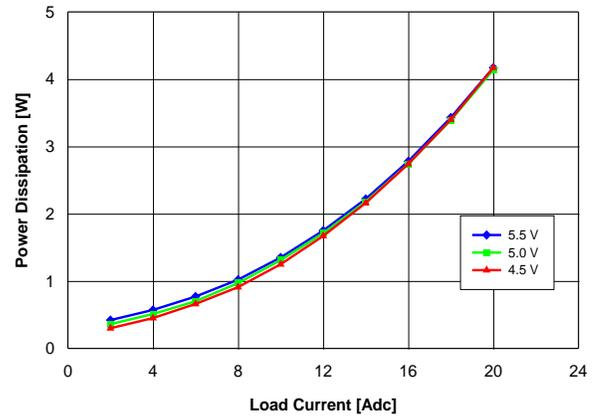
Fig. 2.0V.4: Power loss vs. load current and input voltage for  $V_{out} = 2.0\text{ V}$  converter mounted vertically with air flowing from pin 1 and pin 6 to pins 2 – 5 at a rate of 200 LFM (1 m/s) and  $T_a = 25\text{ }^\circ\text{C}$ .
