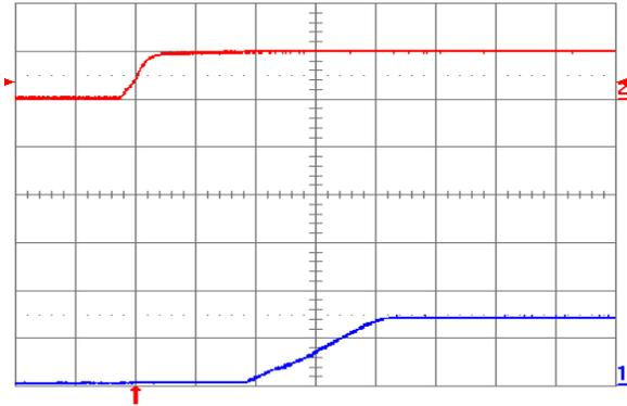
Fig. 1.2V.5: Turn-on transient for  $V_{out} = 1.2\text{ V}$  with application of  $V_{in}$  at full rated load current (resistive) and  $100\text{ }\mu\text{F}$  external capacitance at  $V_{in} = 5\text{ V}$ . Top trace:  $V_{in}$  (5 V/div.); Bottom trace: output voltage (1 V/div.); Time scale: 2 ms/div.
