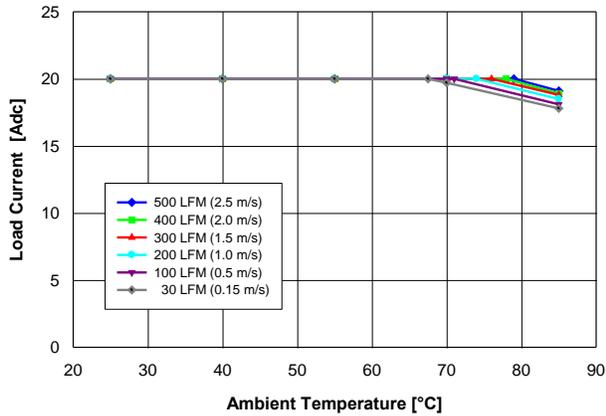
Fig. 1.8V.1: Available load current vs. ambient temperature and airflow rates for  $V_{out} = 1.8\text{ V}$  converter mounted vertically with  $V_{in} = 5\text{ V}$ , air flowing from pin 1 and pin 6 to pins 2 - 5, and maximum MOSFET temperature  $\leq 120^\circ\text{C}$ .
