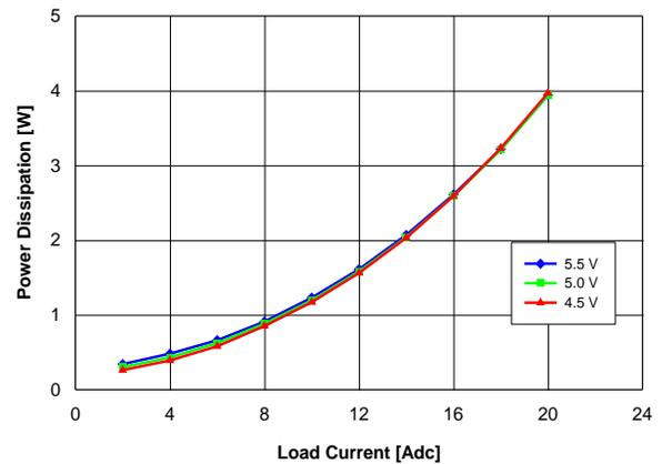
Fig. 1.0V.4: Power loss vs. load current and input voltage for  $V_{out} = 1.0\text{ V}$  converter mounted vertically with air flowing from pin 1 and pin 6 to pins 2 - 5 at a rate of 200 LFM (1 m/s) and  $T_a = 25\text{ }^{\circ}\text{C}$ .
