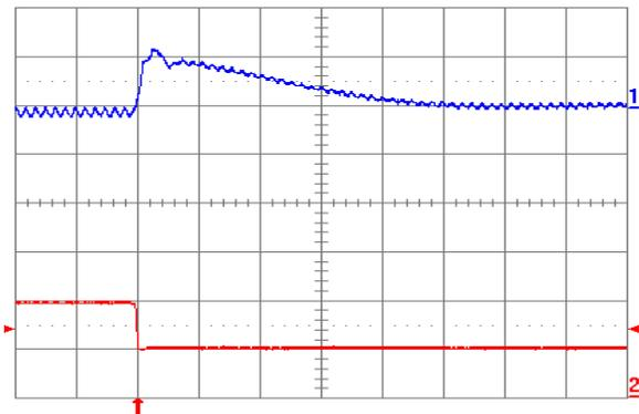
Fig. 1.2V.8: Output voltage response for  $V_{out} = 1.2\text{ V}$  to negative load current step change from 20 A to 10 A with slew rate of  $-5\text{ A}/\mu\text{s}$  at  $V_{in} = 5\text{ V}$ . Top trace: output voltage (100 mV/div.); Bottom trace: load current (10 A/div.).  $C_o = 100\text{ }\mu\text{F}$  ceramic. Time scale: 20  $\mu\text{s}$ /div.
