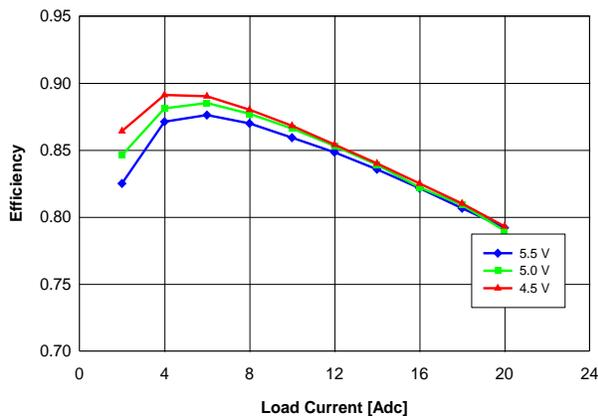
Fig. 0.7525V.3: Efficiency vs. load current and input voltage for  $V_{out} = 0.7525\text{ V}$  converter mounted vertically with air flowing from pin 1 and pin 6 to pins 2 – 5 at a rate of 200 LFM (1 m/s) and  $T_a = 25\text{ }^\circ\text{C}$ .
