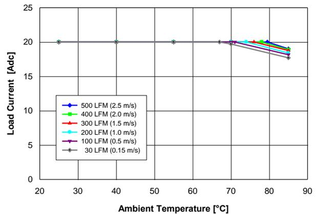
Fig. 2.0V.2: Available load current vs. ambient temperature and airflow rates for  $V_{out} = 2.0\text{ V}$  converter mounted horizontally with  $V_{in} = 5\text{ V}$ , air flowing from pin 1 and pin 6 to pins 2 – 5, and maximum MOSFET temperature  $\leq 120\text{ }^\circ\text{C}$ .
