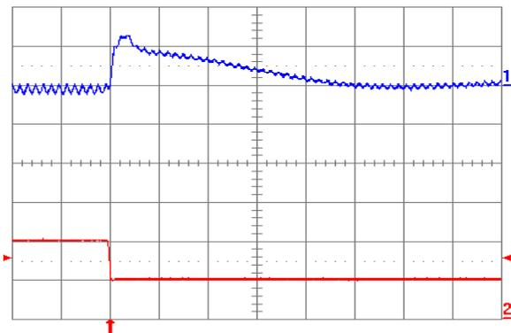
Fig. 2.0V.8: Output voltage response for  $V_{out} = 2.0\text{ V}$  to negative load current step change from 20 A to 10 A with slew rate of  $-5\text{ A}/\mu\text{s}$  at  $V_{in} = 5\text{ V}$ . Top trace: output voltage (100 mV/div.); Bottom trace: load current (10 A/div.).  $C_o = 100\text{ }\mu\text{F}$  ceramic. Time scale: 20  $\mu\text{s}$ /div.
