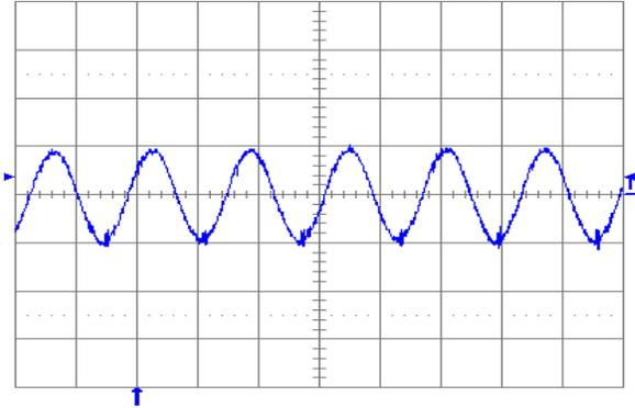
Fig. 1.5V.6: Output voltage ripple (20 mV/div.) at full rated load current into a resistive load with external capacitance  $100\ \mu\text{F}$  ceramic +  $1\ \mu\text{F}$  ceramic and  $V_{in} = 5\text{ V}$  for  $V_{out} = 1.5\text{ V}$ . Time scale: 2  $\mu\text{s}$ /div.
