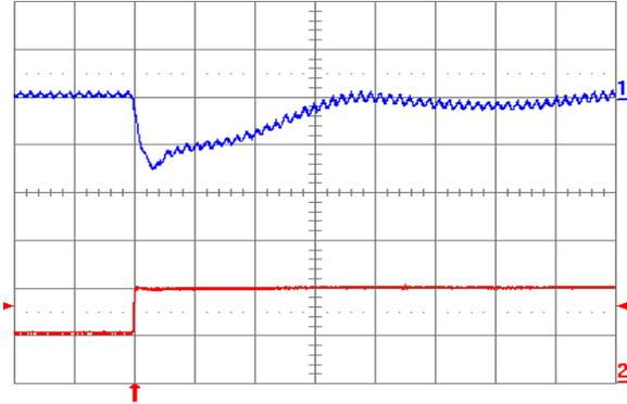
Fig. 3.3V.7: Output voltage response for  $V_{out} = 3.3\text{ V}$  to positive load current step change from 10 A to 20 A with slew rate of  $5\text{ A}/\mu\text{s}$  at  $V_{in} = 5\text{ V}$ . Top trace: output voltage (100 mV/div.); Bottom trace: load current (10 A/div.).  $C_o = 100\text{ }\mu\text{F}$  ceramic. Time scale:  $20\text{ }\mu\text{s}/\text{div}$ .
