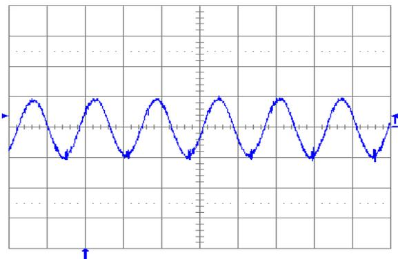
Fig. 1.0V.6: Output voltage ripple (20 mV/div.) at full rated load current into a resistive load with external capacitance  $100\text{ }\mu\text{F}$  ceramic +  $1\text{ }\mu\text{F}$  ceramic and  $V_{in} = 5\text{ V}$  for  $V_{out} = 1.0\text{ V}$ . Time scale: 2  $\mu\text{s}$ /div.
