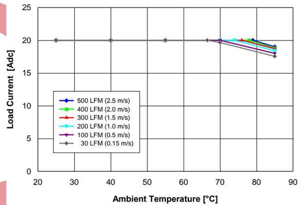
Fig. 2.5V.2: Available load current vs. ambient temperature and airflow rates for  $V_{out} = 2.5\text{ V}$  converter mounted horizontally with  $V_{in} = 5\text{ V}$ , air flowing from pin 1 and pin 6 to pins 2 – 5, and maximum MOSFET temperature  $\leq 120\text{ }^\circ\text{C}$ .
