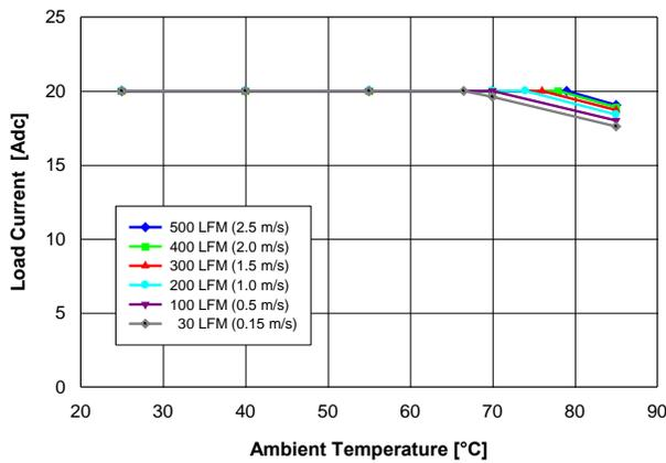
Fig. 2.5V.1: Available load current vs. ambient temperature and airflow rates for  $V_{out} = 2.5\text{ V}$  converter mounted vertically with  $V_{in} = 5\text{ V}$ , air flowing from pin 1 and pin 6 to pins 2 – 5, and maximum MOSFET temperature  $\leq 120\text{ }^\circ\text{C}$ .
