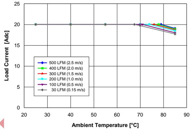
Fig. 1.8V.2: Available load current vs. ambient temperature and airflow rates for  $V_{out} = 1.8\text{ V}$  converter mounted horizontally with  $V_{in} = 5\text{ V}$ , air flowing from pin 1 and pin 6 to pins 2 - 5, and maximum MOSFET temperature  $\leq 120^\circ\text{C}$ .
