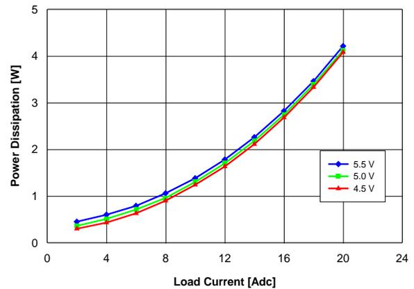
Fig. 3.3V.4: Power loss vs. load current and input voltage for  $V_{out} = 3.3\text{ V}$  converter mounted vertically with air flowing from pin 1 and pin 6 to pins 2 - 5 at a rate of 200 LFM (1 m/s) and  $T_a = 25\text{ }^{\circ}\text{C}$ .
