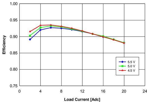
Fig. 1.5V.3: Efficiency vs. load current and input voltage for  $V_{out} = 1.5\text{ V}$  converter mounted vertically with air flowing from pin 1 and pin 6 to pins 2 – 5 at a rate of 200 LFM (1 m/s) and  $T_a = 25^\circ\text{C}$ .
