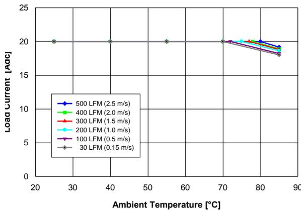
Fig. 0.7525V.1: Available load current vs. ambient temperature and airflow rates for  $V_{out} = 0.7525\text{ V}$  converter mounted vertically with  $V_{in} = 5\text{ V}$ , air flowing from pin 1 and pin 6 to pins 2 – 5, and maximum MOSFET temperature  $\leq 120\text{ }^\circ\text{C}$ .
