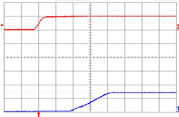
Fig. 1.0V.5: Turn-on transient for  $V_{out} = 1.0\text{ V}$  with application of  $V_{in}$  at full rated load current (resistive) and  $100\text{ }\mu\text{F}$  external capacitance at  $V_{in} = 5\text{ V}$ . Top trace:  $V_{in}$  (5 V/div.); Bottom trace: output voltage (1 V/div.); Time scale: 2 ms/div.
