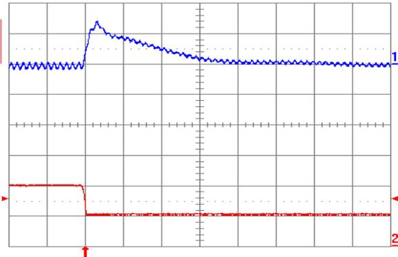
Fig. 2.5V.8: Output voltage response for  $V_{out} = 2.5\text{ V}$  to negative load current step change from 20 A to 10 A with slew rate of  $-5\text{ A}/\mu\text{s}$  at  $V_{in} = 5\text{ V}$ . Top trace: output voltage (100 mV/div.); Bottom trace: load current (10 A/div.).  $C_o = 100\ \mu\text{F}$  ceramic. Time scale: 20  $\mu\text{s}$ /div.
