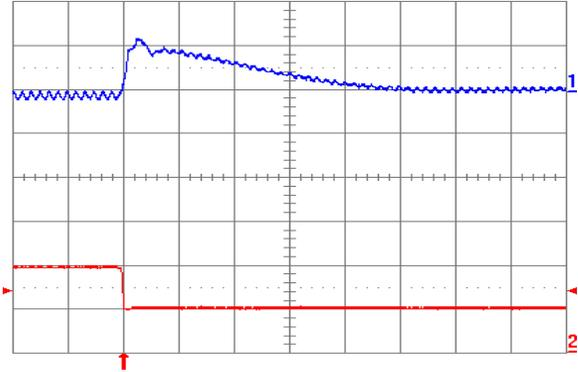
Fig. 1.0V.8: Output voltage response for  $V_{out} = 1.0\text{ V}$  to negative load current step change from 20 A to 10 A with slew rate of  $-5\text{ A}/\mu\text{s}$  at  $V_{in} = 5\text{ V}$ . Top trace: output voltage (100 mV/div.); Bottom trace: load current (10 A/div.).  $C_o = 100\ \mu\text{F}$  ceramic. Time scale:  $20\ \mu\text{s}/\text{div}$ .
