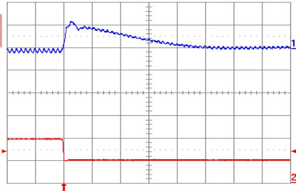
Fig. 1.5V.8: Output voltage response for  $V_{out} = 1.5\text{ V}$  to negative load current step change from 20 A to 10 A with slew rate of  $-5\text{ A}/\mu\text{s}$  at  $V_{in} = 5\text{ V}$ . Top trace: output voltage (100 mV/div.); Bottom trace: load current (10 A/div.).  $C_o = 100\ \mu\text{F}$  ceramic. Time scale: 20  $\mu\text{s}$ /div.
