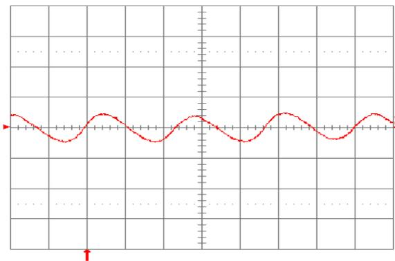
Fig. 15: Input reflected ripple current,  $i_c$  (100 mA/div.), measured at input terminals at full rated load current and  $V_{in} = 24 \text{ V}$ . Refer to Fig. 14 for test setup. Time scale:  $1 \mu\text{s}/\text{div}$ .
