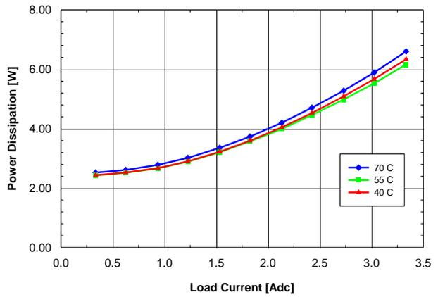
Fig. 8: Power dissipation vs. load current and ambient temperature for SQ24T/S03150 converter mounted vertically with  $V_{in} = 24\text{ V}$  and air flowing from pin 3 to pin 1 at a rate of 200 LFM (1.0 m/s).
