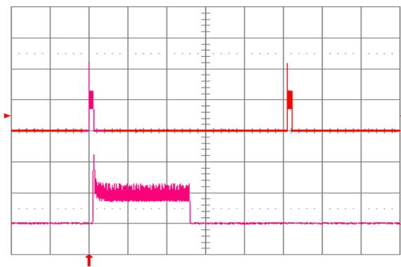
Fig. 18: Load current (top trace,  $5 \text{ A}/\text{div}$ .,  $20 \text{ ms}/\text{div}$ .) into a  $10 \text{ m}\Omega$  short circuit during restart, at  $V_{in} = 24 \text{ V}$ . Bottom trace ( $5 \text{ A}/\text{div}$ .,  $1 \text{ ms}/\text{div}$ .) is an expansion of the on-time portion of the top trace.
