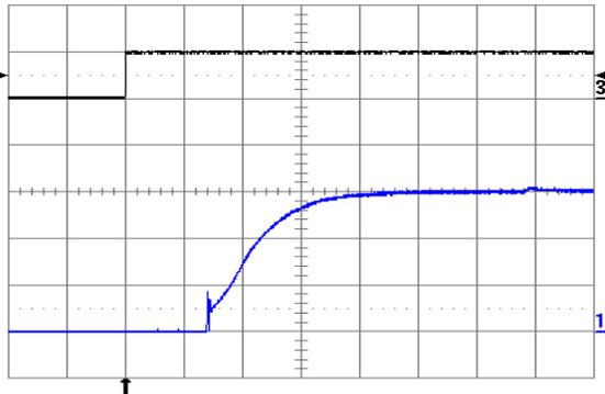
Fig. 9: Turn-on transient at full rated load current (resistive) with no output capacitor at  $V_{in} = 24\text{ V}$ , triggered via ON/OFF pin. Top trace: ON/OFF signal (5 V/div.). Bottom trace: output voltage (5 V/div.). Time scale: 1 ms/div.
