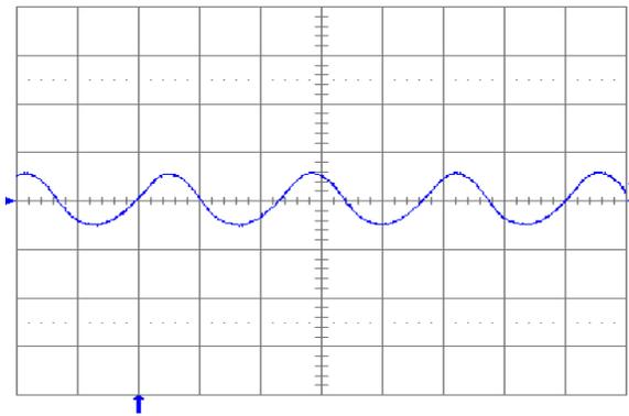
Fig. 13: Output voltage ripple (100 mV/div.) at full rated load current into a resistive load with  $C_o = 10 \mu\text{F}$  tantalum +  $1 \mu\text{F}$  ceramic and  $V_{in} = 24 \text{ V}$ . Time scale:  $1 \mu\text{s}/\text{div}$ .
