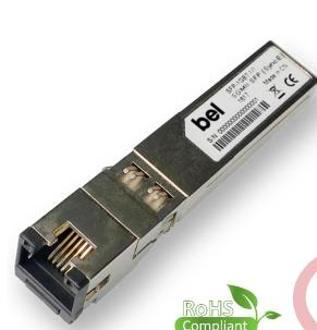
The Bel SFP-1GBT-10 transceiver is a 10/100/1000Base-T SFP module with Synchronous Ethernet capability for SGMII host interface. The host interface transmits and receives serial data differentially at 1.25Gbps. The copper interface is advertised as full duplex and will auto-negotiate to 10/100/1000 Base-T.
