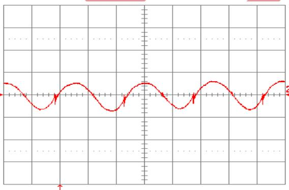
Figure 22. Input reflected ripple current,  $i_c$  (100 mA/div), measured at input terminals at full rated load current and  $V_{in} = 24$  V. Refer to Fig. 21 for test setup. Time scale:  $1$   $\mu$ s/div.
