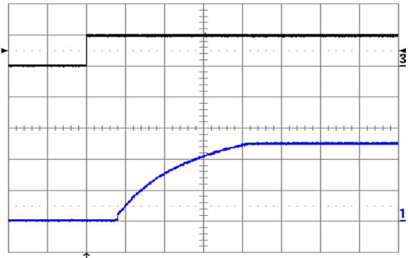
Figure 17. Turn-on transient at full rated load current (resistive) plus 10,000 F at  $V_{in} = 24\text{ V}$ , triggered via ON/OFF pin. Top trace: ON/OFF signal (5 V/div.). Bottom trace: output voltage (2 V/div.) Time scale: 2 ms/div.
