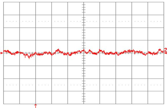
Figure 23. Input reflected ripple current,  $i_s$  (10 mA/div), measured through  $10$   $\mu$ H at the source at full rated load current and  $V_{in} = 24$  V. Re-fer to Fig. 23 for test setup. Time scale:  $1$   $\mu$ s/div.
