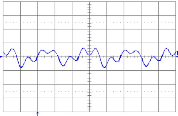
Figure 20. Output voltage ripple (20 mV/div.) at full rated load current into a resistive load with  $C_o = 10$   $\mu$ F tantalum +  $1\mu$ F ceramic and  $V_{in} = 24$  V. Time scale:  $1$   $\mu$ s/div.
