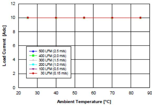
Fig. 1.8V.2: Available load current vs. ambient temperature and airflow rates for YNL05S10018 converter mounted horizontally with  $V_{in} = 5$  V, and maximum MOSFET temperature  $\leq 110$  °C.
