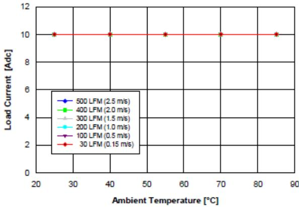
Fig. 3.3V.2: Available load current vs. ambient temperature and airflow rates for YNL05S10033 converter mounted horizontally with  $V_{in} = 5$  V, and maximum MOSFET temperature  $\leq 110$  °C.
