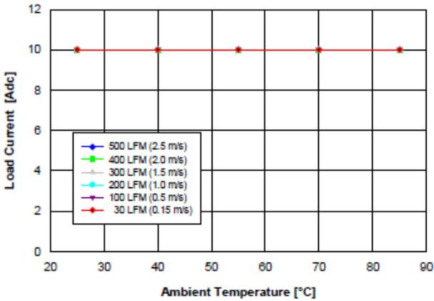
Fig. 1.0V.2: Available load current vs. ambient temperature and airflow rates for YNL05S10010 converter mounted horizontally with  $V_{in} = 5\text{ V}$ , and maximum MOSFET temperature  $\leq 110\text{ }^{\circ}\text{C}$ .
