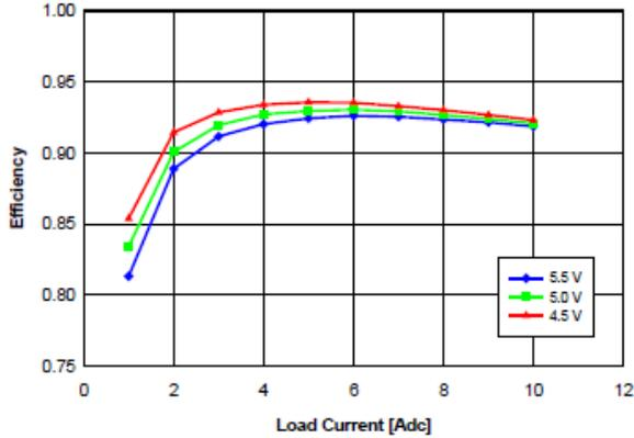
Fig. 2.0V.4: Efficiency vs. load current and input voltage for YNL05S10020 converter mounted vertically with air flowing at a rate of 200 LFM (1 m/s) and  $T_a = 25^\circ\text{C}$ .
