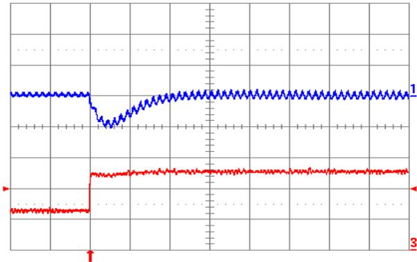
Fig. 1.0V.8: Output voltage response (YNL05S10010) to negative load current step change from 10 A to 5 A with slew rate of -5 A/ $\mu$ s at  $V_{in} = 5$  V. Top trace: output voltage (100 mV/div.); Bottom trace: load current (5 A/div.).  $C_o = 47 \mu$ F ceramic + 1  $\mu$ F ceramic. Time scale: 20  $\mu$ s/div.
