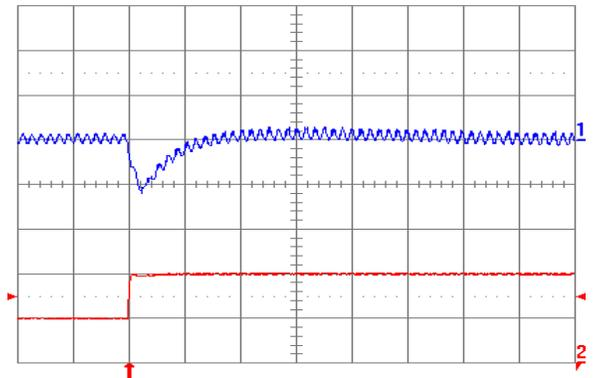
Fig. 3.3V.8: Output voltage response (YNL05S10033) to negative load current step change from 10 A to 5 A with slew rate of -5 A/ $\mu$ s at  $V_{in} = 5$  V. Top trace: output voltage (100 mV/div.); Bottom trace: load current (5 A/div.).  $C_o = 47 \mu$ F ceramic + 1  $\mu$ F ceramic. Time scale: 20  $\mu$ s/div.
