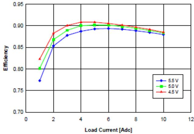
Fig. 1.2V.4: Efficiency vs. load current and input voltage for YNL05S10012 converter mounted vertically with air flowing at a rate of 200 LFM (1 m/s) and  $T_a = 25^\circ\text{C}$ .
