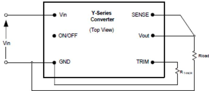
To trim up the output voltage, refer to Fig. E. A trim resistor,  $R_{T-INCR}$ , should be connected between TRIM pin (Pin 3) and GND pin (Pin 5) with value of:
