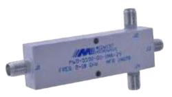
Midwest Microwave's series of high performance isolated Three Way Power Dividers are true three way dividers. They are small, lightweight, ruggedly constructed stripline units that possess inherently low insertion loss and VSWR with high isolation and excellent phase and amplitude tracking. Units are available in ultra-wideband frequency bandwidths covering the entire range of 2.0 - 18.0 GHz.
