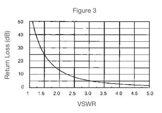
Couplers to be extremely useful in measuring VSWR. Reflectometer test methods utilize this characteristic of directional couplers. The relationship between return loss (dB) and VSWR is shown in figure 3.
