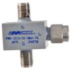
Midwest Microwave's series of Resistive Two Way Power Dividers are very broadband devices that are small, lightweight, ruggedly constructed units that possess consistent VSWR and insertion loss. They also exhibit excellent phase and amplitude tracking. Units are available in wideband frequency bandwidths covering the range of DC - 12.4 GHz and DC - 18.0 GHz.
