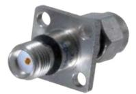
Midwest Microwave's SMA subminiature series of flanged fixed coaxial attenuators (MINIPAD) provide temperature stable, ruggedly built, precision performance in a compact lightweight package size. Attenuation values of 1, 2, 3, 4, 5, 10, and 20 dB are available as standard for both male-female and female-female models.
