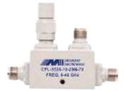
Midwest Microwave 40 GHz directional couplers are small, lightweight, and ruggedly built. They cover a wide bandwidth of 6-40 GHz with low insertion loss and low VSWR. Directional couplers incorporate strip line design with high directivity. They use 2.92mm female stainless-steel interface and are built in aluminum housing coated with gray paint.
