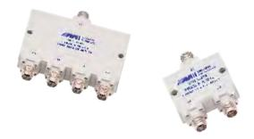
Midwest Microwave 40 GHz power dividers are small, lightweight, and ruggedly built. They cover a wide bandwidth of 6-40 GHz with low insertion loss and low VSWR. Power dividers use Wilkinson design for the lowest insertion loss and the highest isolation. They use 2.92mm female stainless-steel interface and are built in aluminum housing coated with gray paint.
