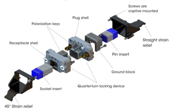
Detailed view of receptacle and plug with accessories for the C-ENX B1 connector.
