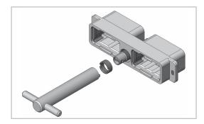
Jackscrews are installed in plugs and jacknuts in receptacle shells. Operator must lock the polarizing device at 1.2 Nm (10.62 Lb-In ) for metallic shell and 0.8Nm (7.08 Lb-In ) for composite shell. Use LOCTITE® 272 to assemble hardware components.
