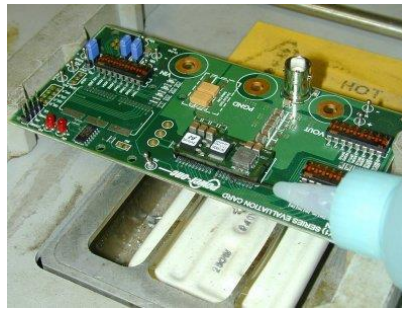
Figure 6: Inject Liquid flux
