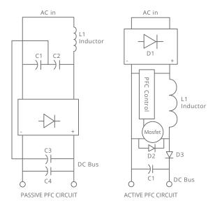
Because of this, it is the strategy that is most widely applied in present-day designs. A switching pre-regulator stage is placed in the input current path of the supply. That regulator is designed not only to maintain a constant dc voltage to feed the main converter stage of the power supply, but also to draw current from the input in-phase with the incoming ac voltage waveform.
