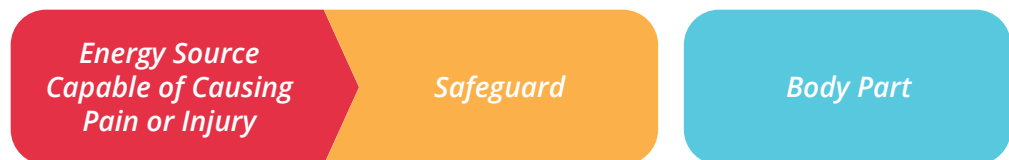
Figure 2: The HBSE three-block model allows a flexible approach to the design of safety features
