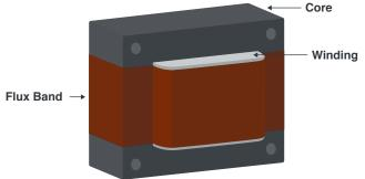
In extreme cases where Power Transformer EMI levels are high, interference can be controlled by using a magnetic shielding enclosure. Such enclosure surrounds the transformer, captures stray magnetic flux or EM radiation and channels unwanted energy to a ground plane. These enclosures unfortunately add cost, weight and manufacturing complexity. They should be used only in cases where EMI from the transformer is excessive and cannot be isolated by any other means.
