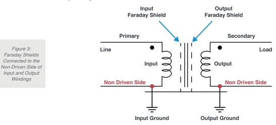
In low power transformer designs a Faraday shield can be eliminated by the use of a splitbobbin where input and output windings are wound non-concentric in separated cavities totally isolated from one another. The space between the input and output windings reduces the inter-winding capacitance, the capacitive coupling and so a decrease in CM noise occurs.
