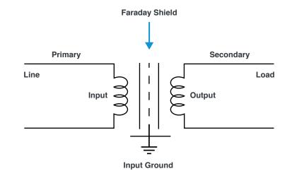
Output windings of Power Transformers can also transfer EM energy via capacitive coupling to the input windings. To mitigate this effect, some transformer designs use another Faraday shield wrapped around the output windings and connected to the Output Ground.
