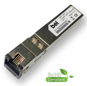
The Bel SFP-1GBT-10 transceiver is a 10/100/1000Base-T SFP module with Synchronous Ethernet capability for SGMII host interface. The host interface transmits and receives serial data differentially at 1.25 Gbps. The  $\,$ copper interface is advertised as full duplex and will auto-negotiate to 10/100/1000 Base-T.
