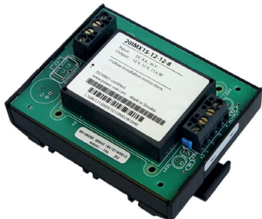
Fig. 24 DIN-rail mounting support HZZ00628-G (previously DMBIMX15)
