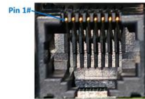
Figure 11. Signal Connector Pin Out (8P8C Modular Jack)
