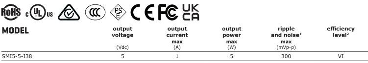
Notes: 1. At full load, nominal Vac input, 25 °C, 20 MHz bandwidth oscilloscope, each output terminated with 0.1 µF and 10 µF capacitors. 2. CoC Tier 2 compliant
