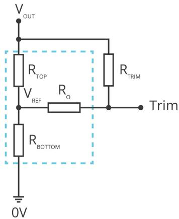
$$R_{\text{TRIM}} = \frac{a \cdot R_{\text{BOTTOM}}}{R_{\text{BOTTOM}} - a} - R_o$$
